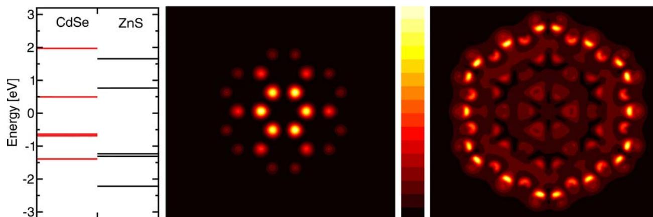
**Figure 3** Cross-section views of the charge distribution of the CBM electron state and VBM hole state in core-shell nanorods. The atomic structure is that of rod III in Fig. 1.
