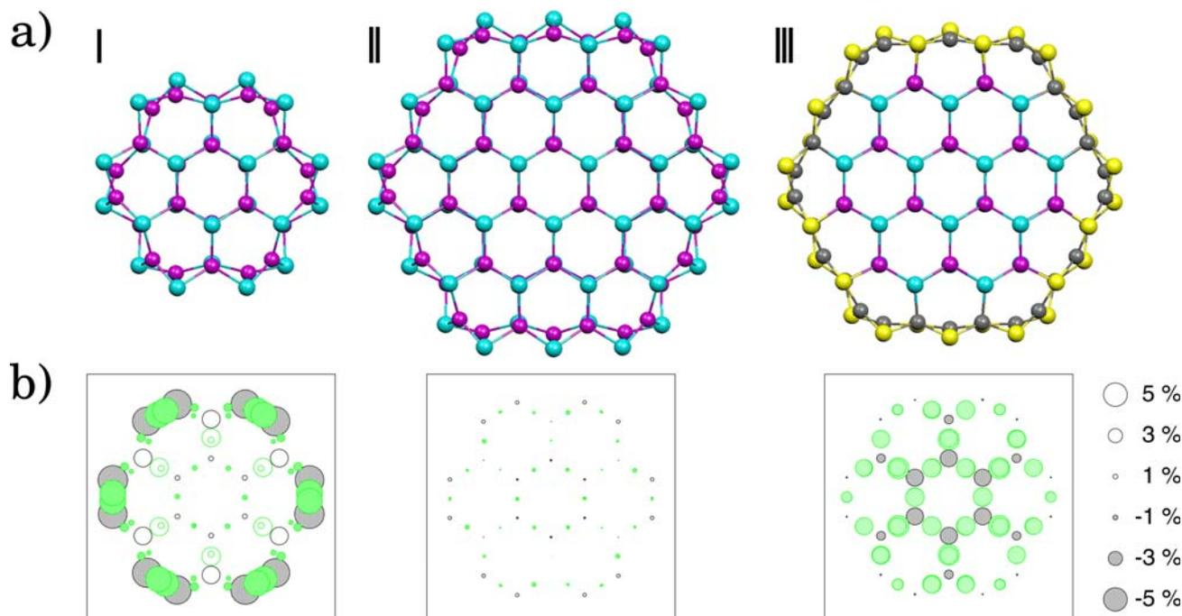
**Figure 1** Cross sections of the CdSe nanorods (upper row) and bond length deviations compared to bulk CdSe (lower row).
