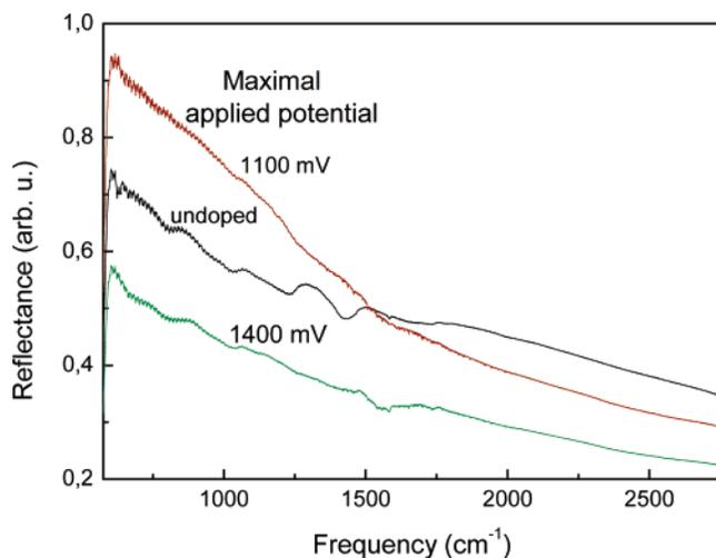
**Figure 4.** Far-IR reflectance spectra of SWNT samples polarized to different maximal potentials in 1 M KCl.
