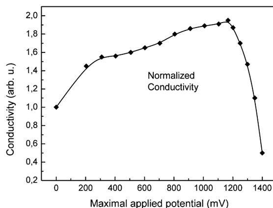
**Figure 3.** Normalized dc conductivity of the SWNT working electrode vs maximal applied potential in 1 M KCl. The displayed values are normalized to the conductivity of the undoped sample.
