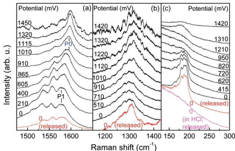
**Figure 1.** Raman spectra at 1.92 eV excitation energy of the high-energy mode (HEM) (a), the disorder-induced (D) mode (b), and the radial breathing mode (RBM) (c) at several elevated potentials in 1 M KCl. The red traces marked with “released” were obtained after releasing the applied potential from its maximal value down to 0 mV. The lowest trace in (c) was obtained after releasing the potential to 0 mV in 1 M HCl.
