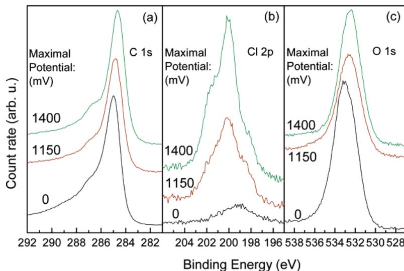
**Figure 5.** XPS spectra of the carbon 1s (a), chlorine 2p (b), and oxygen 1s (c) level in SWNT samples polarized to different maximal potentials in 1 M HCl as quoted in the graphs.  $U_{\max} = 0$  mV means only a brief wetting of the sample in the solution without electrical contact.
