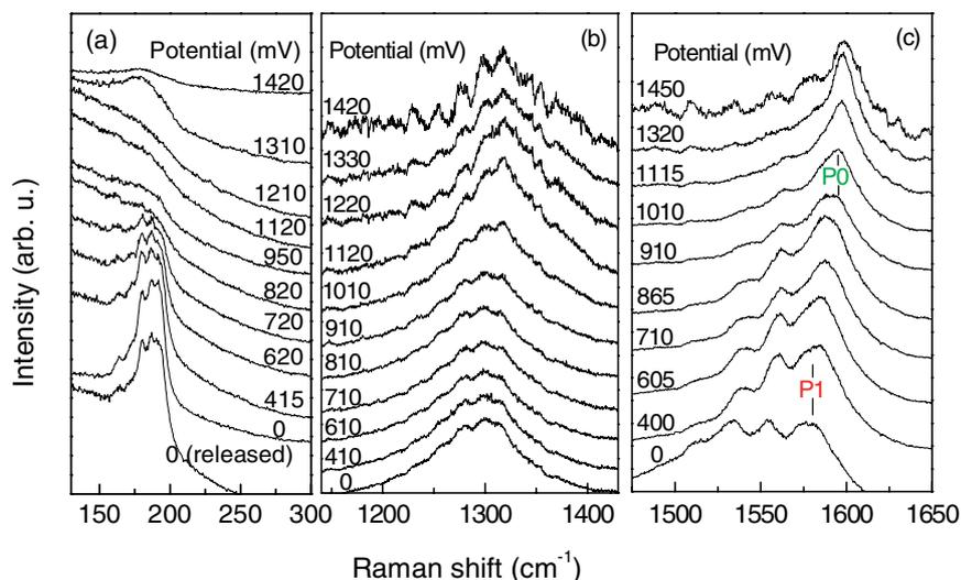
**Fig. 1** (online colour at: [www.pss-b.com](http://www.pss-b.com)) Raman spectra at 1.92 eV excitation energy of the radial breathing mode (a), the disorder-induced mode (b) and the high-energy mode (c) at several elevated potentials.
