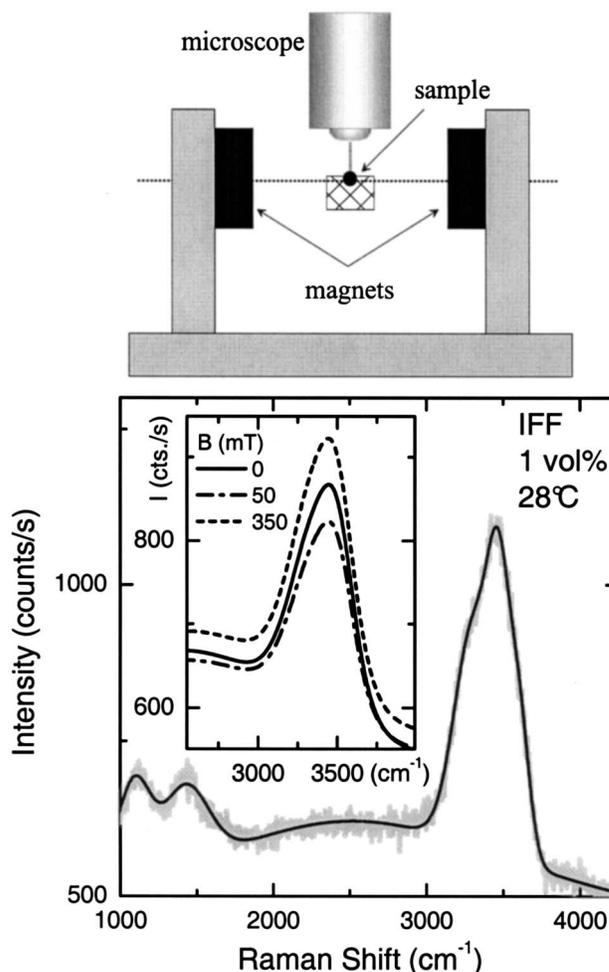
FIG. 1. Upper panel: Sketch of the experimental setup in cross section along the magnetic-field axis. Lower panel: Representative Raman spectrum of a 1 vol % aqueous ionic ferrofluid (IFF) measured at 28 °C and zero magnetic field. The solid curve represents a line-shape fitting function (see text for details). The inset shows three spectra in the energy region of the water stretching mode for different magnetic fields.
