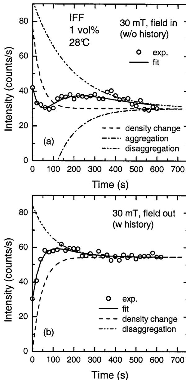
FIG. 3. Time dependence of the integrated intensity of the OH Raman band (open circles) for a 1 vol% IFF at 28 °C when a field of 30 mT is (a) suddenly switched on or (b) switched off. Solid curves are fits to the data points using different exponential functions corresponding to the processes of (dashed line) change in the density of nanoparticles, (dash-dotted line) aggregation, and (dash-double-dotted line) disaggregation.
