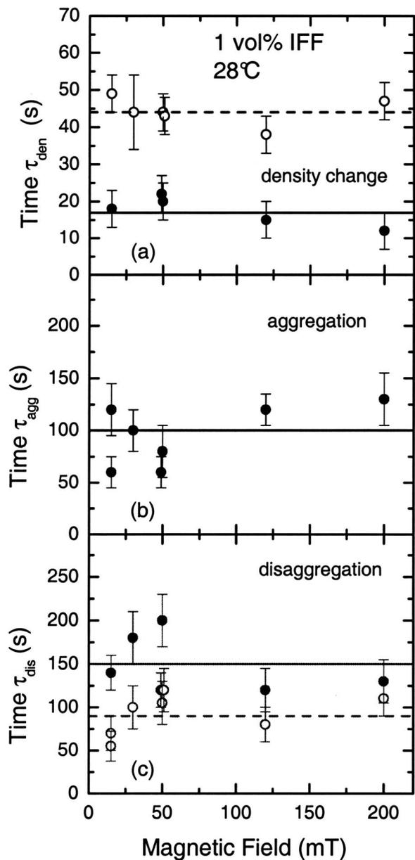
FIG. 5. Time constants as a function of external magnetic field for a 1 vol % IFF at 28 °C corresponding to the processes of (a) change in particle density, (b) aggregation into clusters, and (c) disaggregation of clusters, as determined from fits to the transients of Fig. 4 using exponential functions. Horizontal solid and dashed lines represent the mean values of the time constants corresponding to each process upon switching on (full symbols) and off (open circles) the field, respectively.
