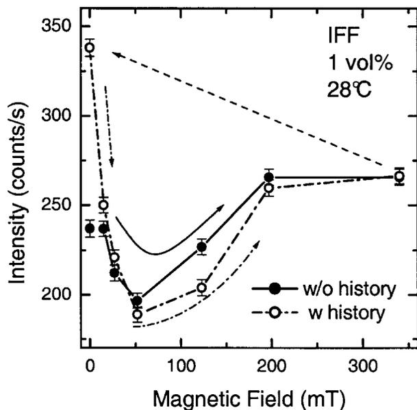
FIG. 2. Raman intensity of the water stretching mode as a function of magnetic field at 28 °C for the cases with (open symbols/dashed line) and without (full symbols and line) previous magnetic-field history. Arrows indicate the sense of variation of the field.
