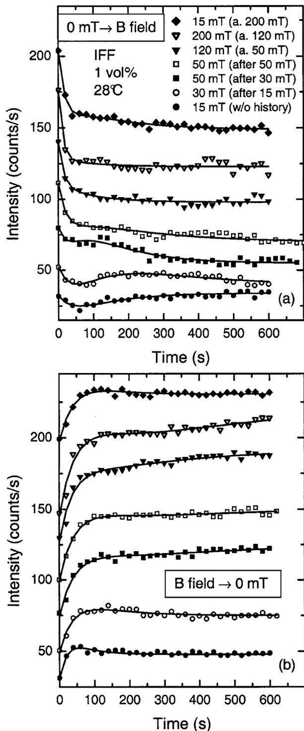
FIG. 4. Time dependence of the integrated intensity of the OH Raman band (symbols) for a 1 vol% IFF at 28 °C for the sudden (a) switching on or (b) switching off of different magnetic fields, as indicated in the legend. Solid curves are fits to the data points using different exponential functions corresponding to the field-induced processes of density change, aggregation, and disaggregation.
