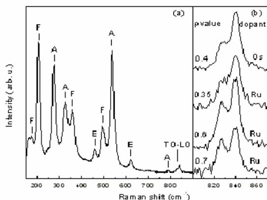
Fig. 3. a) Sample Raman spectrum representative of the spatially-resolved measurements in a Z(XY)Z polarization geometry on the BSO:Ru and BSO:Os crystals. b) Raman spectra of the high-energy antisymmetric stretching BSO mode as measured from the core region of the BSO:Os crystal (upper trace) and the BSO:Ru crystal (all three remaining traces). Note the substantial variation of the TO/LO intensity ratio in the core of the BSO:Ru crystal. The spectra were vertically shifted for clarity.
