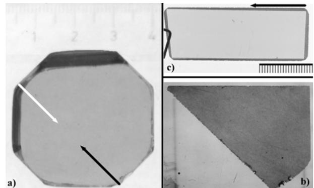
Fig. 2. a) A photograph of the (001) surface of the 8 mm thick BSO:Os wafer. The black arrow marks the [110] direction. b) A XRDTT image of the (001) surface- (006) reflection. c) A photograph of the (110) slice. The marker represents 10 mm.
