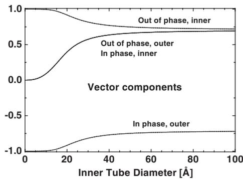
**Fig. 1** Normalized coordinates  $x_j^i$  of the BLMs as function of the inner diameter  $D$ . In the  $D \rightarrow \infty$  limit the values  $\pm 1/\sqrt{2}$  corresponding to the displacements of the graphene transverse acoustic and the  $B_{2g}$  phonon modes ( $127 \text{ cm}^{-1}$ ) are obtained.
