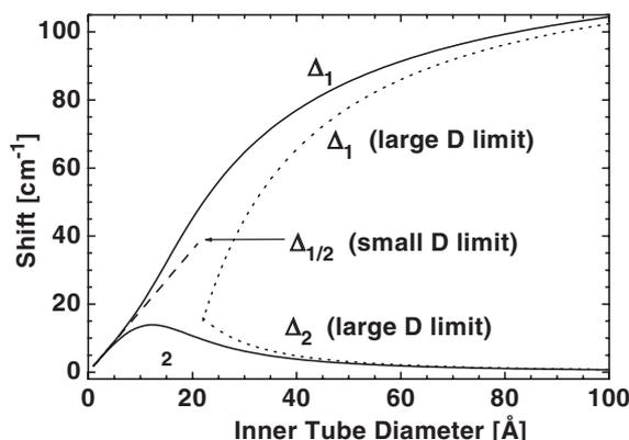
**Fig. 3** The BLMs shifts relative to the corresponding SWCNTs RBMs. The analytic results are obtained directly from (2), while small and large  $D$  limits are given by (4) and (5).
