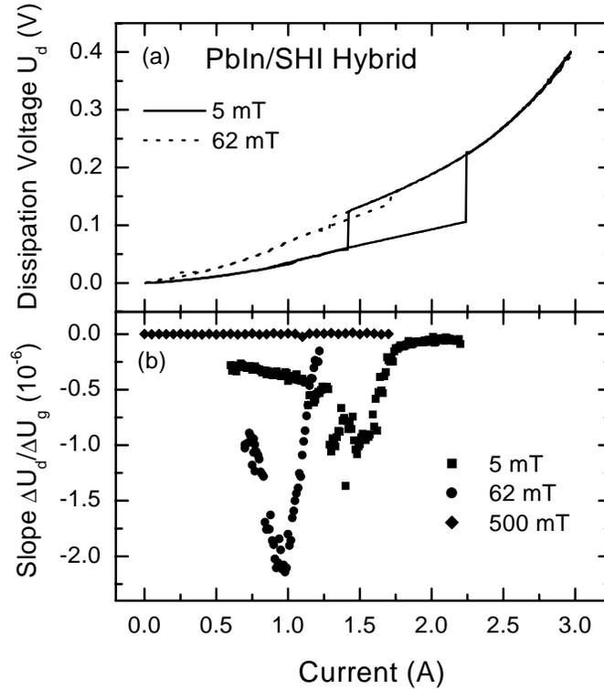
**Figure 3.** (a) Current-voltage characteristics of a 125-nm-thick PbIn/SHI hybrid for 5 and 62 mT at 4.2 K. (b) Dependence on transport current of the slope of the straight line obtained from the  $U_d$ -versus- $U_g$  curves, as shown in the Inset to Fig. 2, for different magnetic fields.
