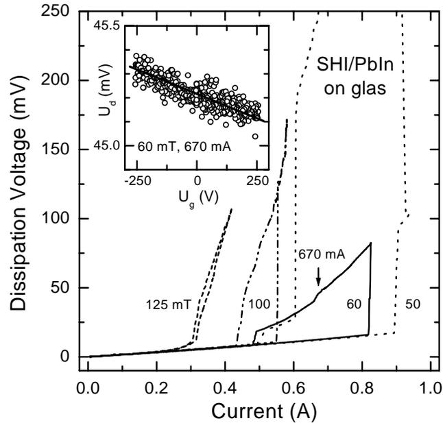
**Figure 1.** Current-voltage characteristic of a PbIn film pressed on a GaAs single heterointerface (SHI) structure for different magnetic fields. The inset shows the dissipation voltage ( $U_d$ ) as a function of positive and negative gate voltages ( $U_g$ ). The arrow indicates the position where the  $U_d$ -versus- $U_g$  curve was measured.
