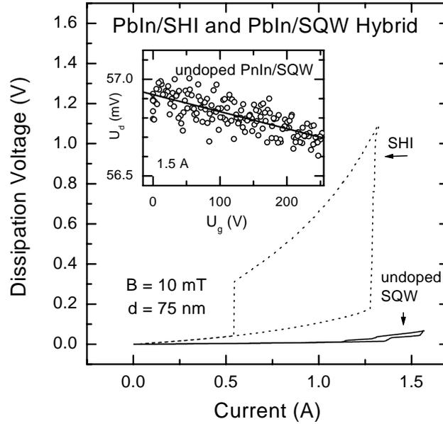
**Figure 2.** Current-voltage characteristic of a PbIn/SHI hybrid (dashed curve) and an one with an undoped SQW structure (solid line) measured at 4.2 K for 10 mT. The inset shows the dissipation voltage ( $U_d$ ) as a function of the gate voltage ( $U_g$ ) for the undoped-SQW hybrid obtained with a superconductor-transport current of 1.5 A.
