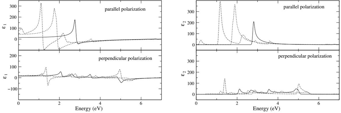
**FIGURE 1.** Dielectric function of the three isolated nanotubes. Left: real part, right: imaginary part. The solid line corresponds to the (3,3) nanotube, the dotted line to the (5,0), and the dashed line to the (4,2).
