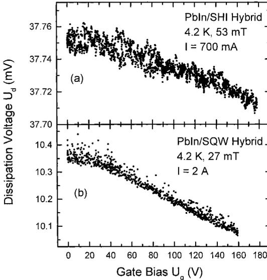
Fig. 3. Dissipation voltage as a function of gate bias of a) a PbIn/SHI and b) a PbIn/SQW hybrid structure at 4.2 K and in a perpendicular magnetic field of 53 and 27 mT using a transport current of 700 mA and 2 A, respectively
