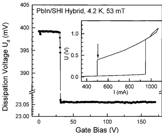
Fig. 4. Dissipation voltage as a function of gate bias of a PbIn/SHI hybrid structure in a perpendicular magnetic field of 53 mT, with 500 mA current and at 4.2 K. The inset shows the corresponding current–voltage characteristic. The point where the measurement of dissipation versus gate voltage was taken is marked with an arrow
