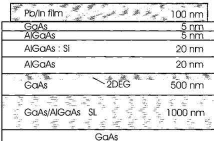
Fig. 1. Cross section of the PbIn/SHI hybrid sample showing the growth sequence. The position at which the electron gas (2DEG) forms, is indicated
