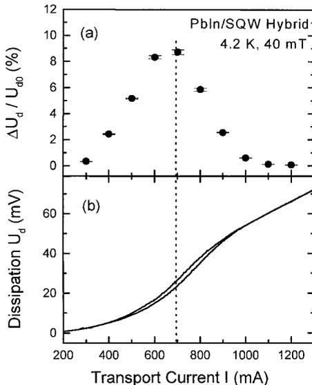
Fig. 5. a) Percentage change in dissipation versus current of a PbIn/SQW hybrid at 4.2 K and 40 mT. The percentage is calculated as the maximum dissipation change in a gate voltage interval of 170 V, divided by the initial dissipation value. b) The corresponding  $I$ - $V$  characteristic; the dashed line marks the position of the damping maximum
