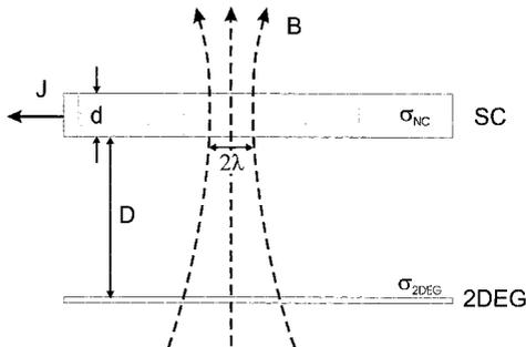
Fig. 2. Schematic representation of the superconductor–2DEG hybrid device. A transport current  $J$  flows through a superconducting film (SC) of thickness  $d$  and normal-state conductivity  $\sigma_{\text{NC}}$ . It couples to a 2DEG at a distance  $D$  through the magnetic field  $B$  of the vortices
