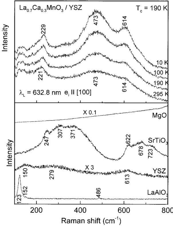
Fig. 2. Raman spectra at different temperatures of a polycrystalline  $\text{La}_{0.7}\text{Ca}_{0.3}\text{MnO}_3$  film with  $T_c = 190$  K deposited on YSZ (top panel). Raman spectra at room temperature of the different substrates (bottom panel). The polarization of incident laser light is along quasi-cubic [100] direction. No analyzer has been used
