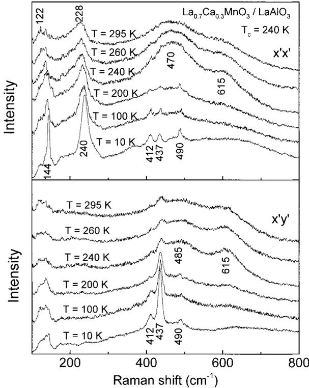
Fig. 1. Polarized Raman spectra at different temperatures of an oriented  $\text{La}_{0.7}\text{Ca}_{0.3}\text{MnO}_3$  film ( $T_c = 240$  K) deposited on  $\text{LaAlO}_3$ . The scattering configurations are indicated on the spectra. The feature at  $122$  to  $144$   $\text{cm}^{-1}$  is due to a leakage from the  $\text{LaAlO}_3$  substrate
