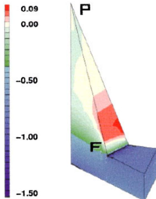
FIG. 3. Mean stress distribution (GPa) inside the pyramid and in the GaN layer.
