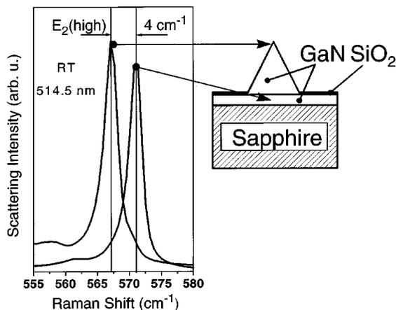
FIG. 2. Raman depth profile at RT. The solid curve represents a spectrum taken from the peak of the pyramid. The spectrum from the  $2 \mu\text{m}$  GaN buffer layer is shown as a dashed curve.
