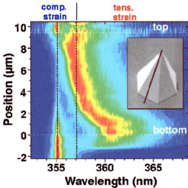
FIG. 1. CL spectrum line scan  $I(s, \lambda)$  at  $T=5^\circ \text{K}$  along a  $\{1\bar{1}01\}$  facet of a pyramid. The white dashed lines mark the top and bottom of the GaN pyramid. The spectral positions of  $(D^0, X)$  emission from the compressively stressed  $2 \mu\text{m}$  GaN layer (355 nm) and the fully relaxed GaN (357.1 nm) are marked by the vertical dotted lines.
