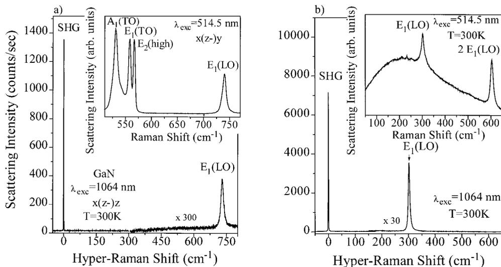
Fig. 1. Room-temperature HR spectra of a) GaN and b) CdS. The insets show Raman spectra taken at room temperature for comparison
