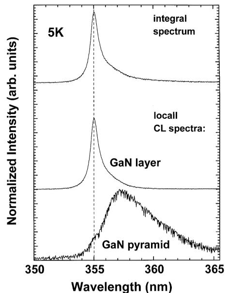
Fig. 1. Local spot-mode CL spectra taken at positions on the GaN pyramid and in between pyramids, compared with a spatially integrated CL spectrum.
