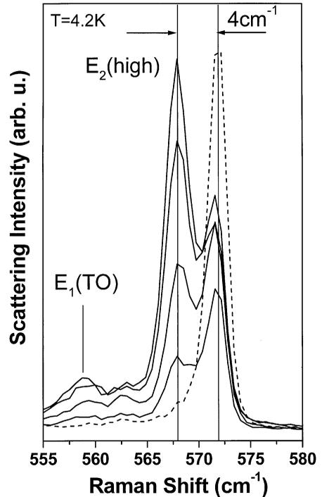
Fig. 3. Raman depth profile at  $T = 4.2$  K. The solid curves represent spectra taken from various depths of the pyramid, the spectra from the  $2\ \mu\text{m}$  GaN epilayer is shown as dashed curve.
