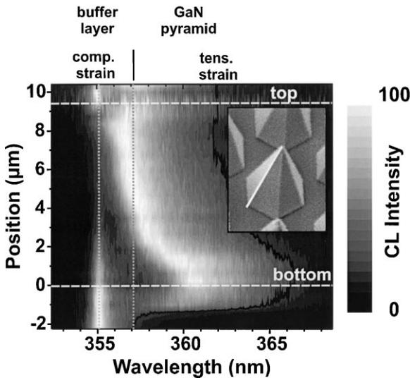
Fig. 4. CL spectrum linescan  $I(\lambda, s)$  at  $T = 5$  K along the edge of a GaN pyramid, indicated as white lines in the SEM-picture (inset). The dashed white lines mark the bottom and top position of the GaN pyramid. The spectral position of  $(D^0, X)$ -emission from the compressively strained  $2\ \mu\text{m}$  GaN layer (355 nm) as well as from the completely relaxed GaN (357.1 nm) are marked by dotted lines.
