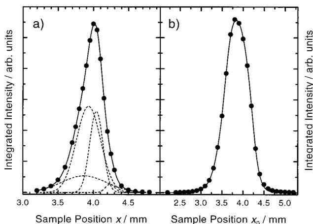
**Figure 2.** (a) Representation (solid line) of the excitation and detection characteristic measured with a 1  $\mu\text{m}$  cubic GaN sample (dots) by a sum of four Gaussian functions (dashed lines). (b) Experimental depth profile of a 1 mm BaF<sub>2</sub> sample (dots) and the result of the model in Eqn (8) (solid line).
