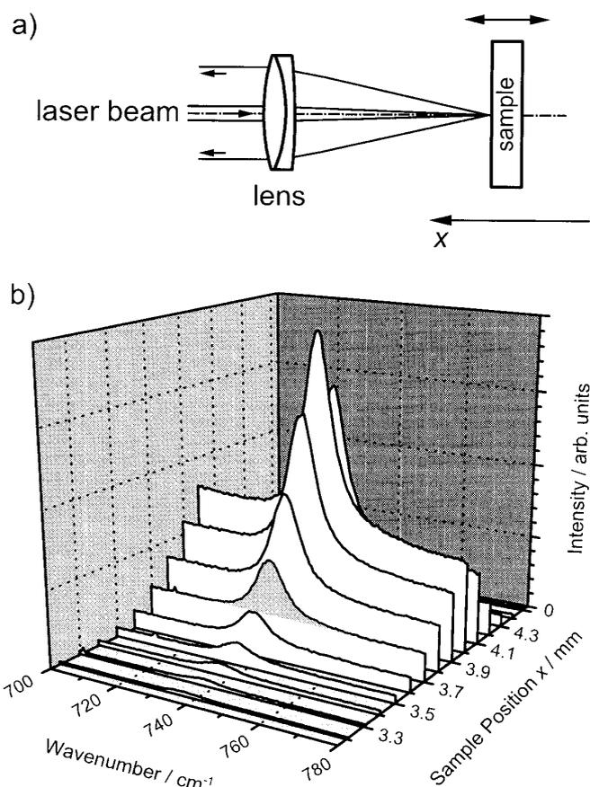
**Figure 1.** (a) Raman spectra recorded in backscattering geometry with the sample being displaced along the optical axis. (b) Series of Raman spectra of cubic GaN (1.25  $\mu\text{m}$  layer) for various sample positions  $x$ .
