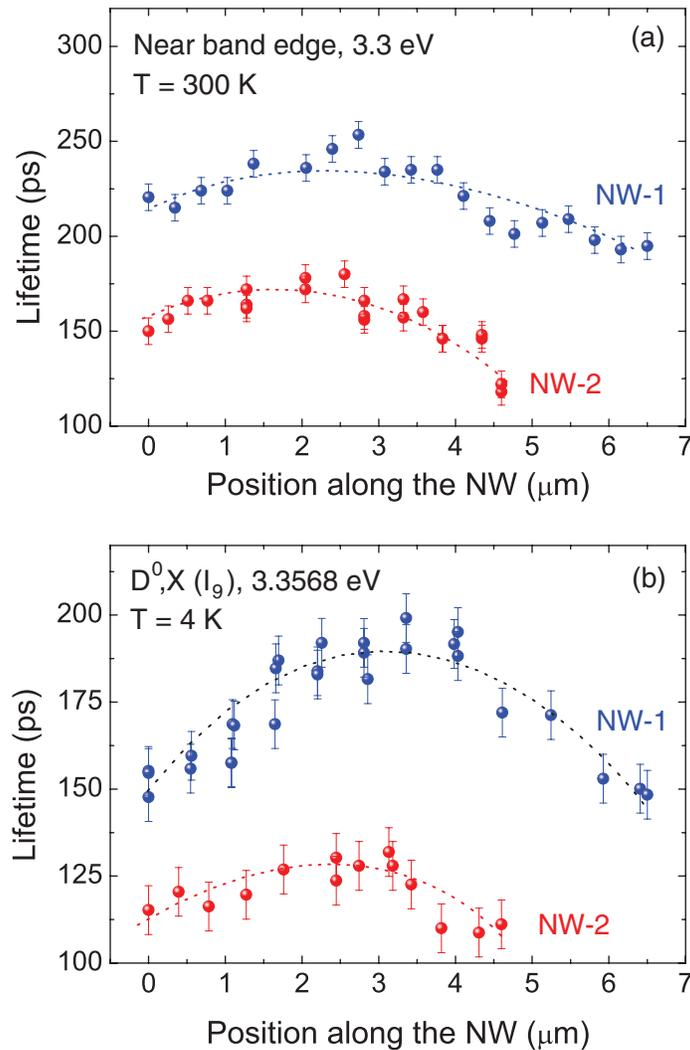
FIG. 3. Spatial dependence of the NBE and DX lifetimes for NW-1 and NW-2. (a) Experimental data for the NBE emission obtained at 300 K, whereas (b) data for the I<sub>9</sub> DX state at 4 K. The dotted lines are guides to the eye.
