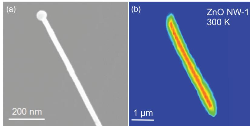
FIG. 1. Single ZnO NW investigated using SEM and  $\mu$ -PL at 300 K. (a) SEM image of a single ZnO NW. The catalyst Au droplet can be clearly observed in the tip of the NW. (b) Integrated  $\mu$ -PL mapscan of NW-1 (false color image max = red, min = blue).
