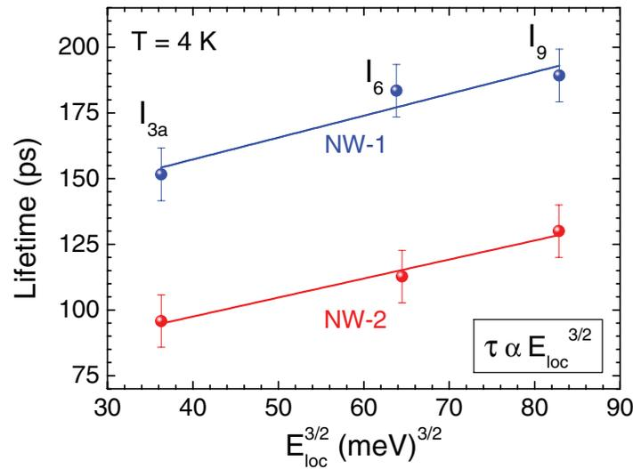
FIG. 4. Donor bound exciton (DX) lifetimes as function of localization energy ( $E_{loc}$ ) to the power of  $3/2$  for NW-1 and NW-2. The observed linear relations are in accordance with the model of Rashba and Gurgenshili.<sup>24</sup> The straight lines represent least-squares fits to the data points.
