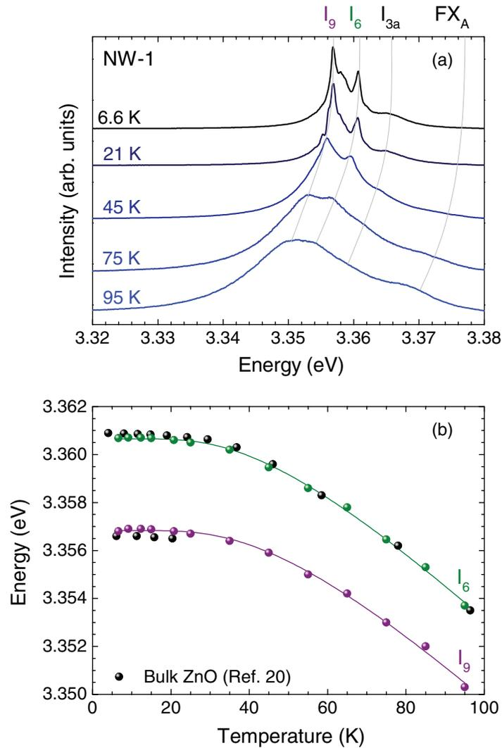
FIG. 2. (a) Temperature dependent  $\mu$ -PL spectrum at the center of NW-1. (b) Temperature dependence of the energy position of the  $I_9$  and  $I_6$  DX transitions in comparison to those of a bulk ZnO substrate. The solid lines represent fits to the data points using the model by Viña *et al.*<sup>29</sup> Error bars are smaller than the symbol's size.
