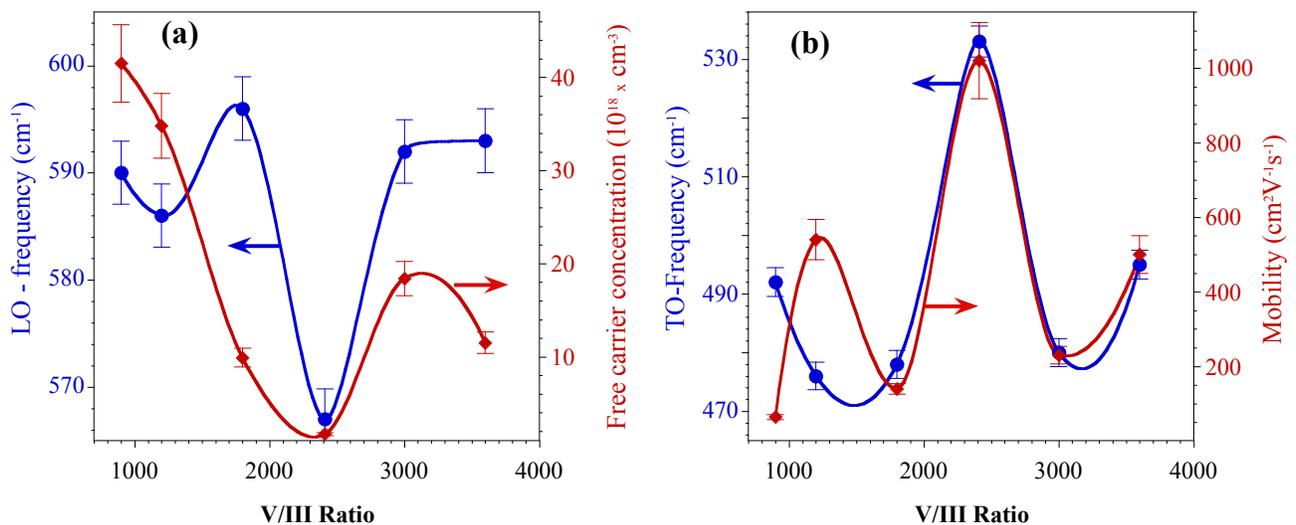
Figure 5. Group V/III molar precursor ratio dependence of the IR reflection. (a)  $\omega_{LO}$  frequency (blue squares, left axis) and free carrier concentration (red circles, right axis) as a function of group V/III precursor ratio. (b)  $\omega_{TO}$  frequency (blue squares, left axis) and mobility (red circles, right axis) as a function of group V/III precursor ratio.
