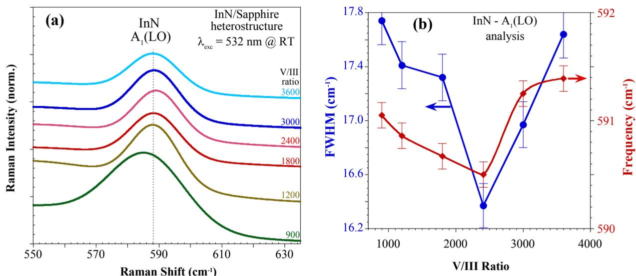
Figure 3. Group V/III molar precursor ratio dependence of the  $A_1(\text{LO})$  phonon mode. (a) Measured Raman spectra for group V/III molar precursor ratio between 900 and 3600 along the (0001) plane. (b) FWHM (blue squares, left axis) and frequency (red circles, right axis) as a function of group V/III molar precursor ratio.
