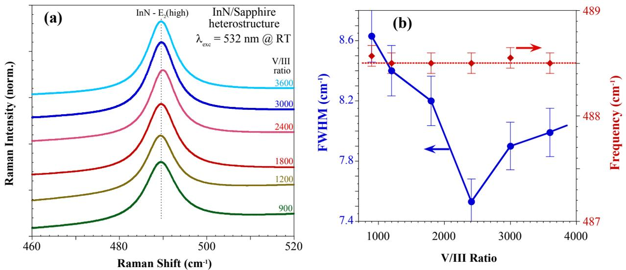
Figure 2. Group V/III molar precursor ratio dependence of the  $E_2(\text{high})$  phonon mode. (a) Measured Raman spectra for group V/III molar precursor ratio between 900 and 3600 along the (0001) plane. (b) FWHM (blue squares, left axis) and frequency (red circles, right axis) as a function of group V/III molar precursor ratio.
