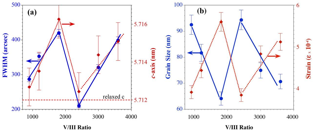
Figure 1. Group V/III molar precursor ratio dependence of the X-ray diffraction ( $2\theta$ - $\omega$ ) TrAx analyses for HPCVD grown InN epilayers. (a) FWHM (left scale) and *c*-axis length (right scale) as a function of V/III ratio. (b) Grain size (left scale) and in-plane strain (right scale) as a function of V/III ratio.
