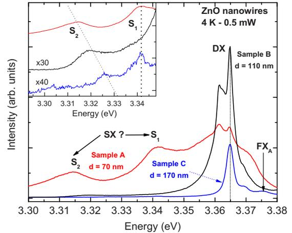
FIG. 2. (Color online) PL spectra at 4 K for samples A, B, and C. The vertical dashed line shows the position of the DX=3.365 eV neutral-bound exciton recombination. The inset shows the detail of the low energy region where two surface related transitions labeled as S<sub>1</sub> and S<sub>2</sub> are observed.
