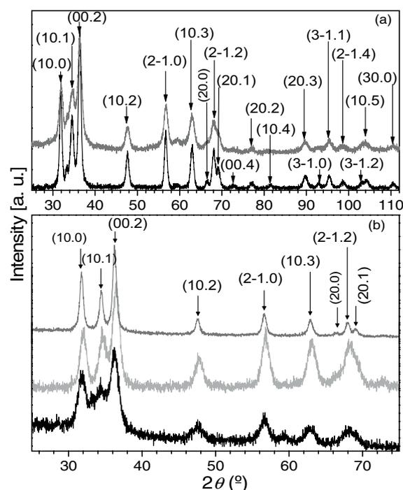
**Figure 2** XRD measurements of (a) ZnO NCs doped with 5% Mn (NC1, black trace) and 10% Mn (NC2, dark gray); (b) ZnO NCs doped with 5% Co (NC3, black), polystyrene capped (NC4, light gray) or ZnSe capped (NC5, dark gray) ZnO:5% Co NCs.
