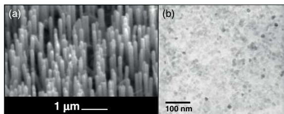
**Figure 1** (a) Typical SEM image of the ZnO nanowires, taken under 45° viewing angle for the nominally 3 at% Mn doped ZnO NWs. (b) Typical TEM image of the ZnO colloidal nanocrystals, taken for the 5 at% doped Mn ZnO NCs.
