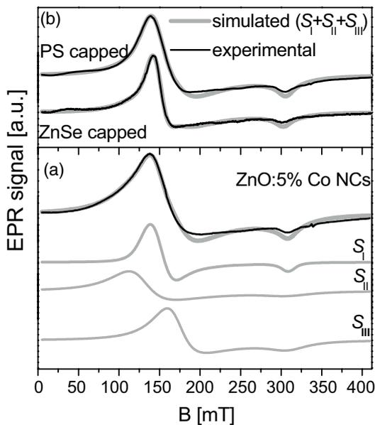
**Figure 5** Experimental EPR spectra (black) measured at 10 K for (a) raw 5% Co doped ZnO NCs (sample NC3) and (b) those capped with polystyrene (PS) (sample NC4) or ZnSe (sample NC5), superimposed with the result of the respective simulation (light gray) given by the sum of the components  $S_I$ ,  $S_{II}$  and  $S_{III}$ .
