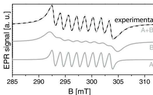
**Figure 4** Experimental EPR spectrum (black) of  $Co^{2+}$  in ZnO NWs (sample NW3), measured at 4.2 K for  $B \parallel c$  ( $\theta = 0^\circ$ ), superimposed with the result of the fitting given by the sum of components A and B (light gray).
