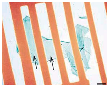
The thinnest material that will ever exist: The arrows point to a monolayer membrane hanging on a scaffold of fine gold wires (marker length: 500 nm) (Figures: MPI-FKF)
