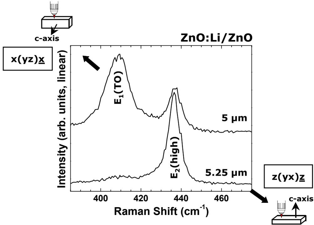
Fig. 7. Raman spectra of Li-doped ZnO grown on ZnO substrate. The spectra were taken at intervals of only 0.25  $\mu\text{m}$  showing a switch between an in-plane (upper curve) and an on-plane (lower curve) configuration.
