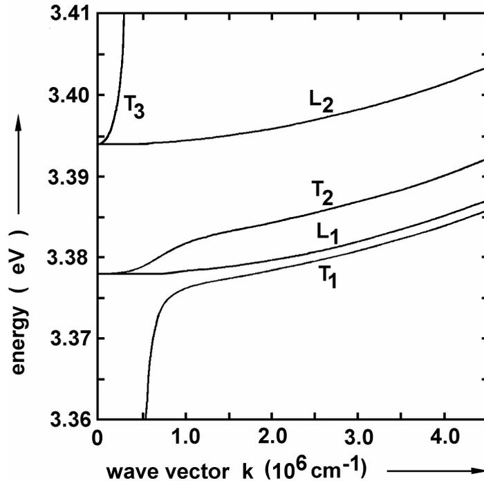
Fig. 3. Dispersion relation of exciton-polaritons in ZnO. The various transversal (T1, T2, T3) and longitudinal (L1, L2) exciton-polariton dispersion curves are shown for a temperature of 2 K.
