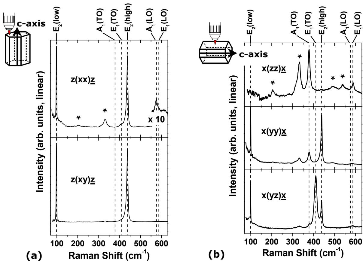
Fig. 5. Room-temperature Raman spectra of a ZnO single crystal taken in different (a) on-plane and (b) in-plane scattering configurations as depicted. Peaks labeled with an asterisk originate from multiphonon scattering.
