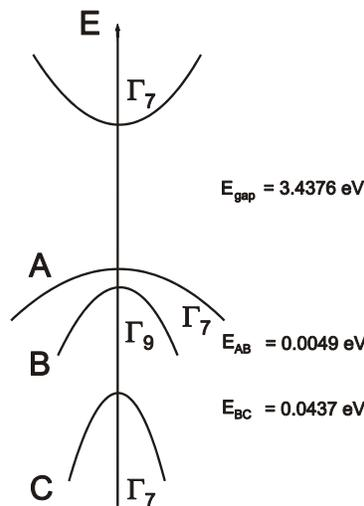
Fig. 1. Splitting of the valence band into the A, B, and C sub-bands with  $\Gamma_7$ ,  $\Gamma_9$ ,  $\Gamma_7$  symmetry caused by the combined effects of crystal-field splitting and spin-orbit coupling. The energy values are indicated for T = 4.2 K.
