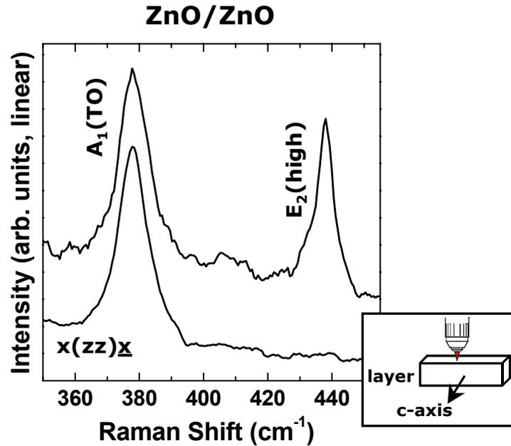
Fig. 6. Room-temperature Raman spectra taken in different depth of an undoped ZnO layer grown on ZnO template. The lower curve shows the shape expected in  $x(zz)x$  configuration (no  $E_2$ -mode), the upper curve illustrates a crystal perturbation (appearance of the forbidden  $E_2$  mode).
