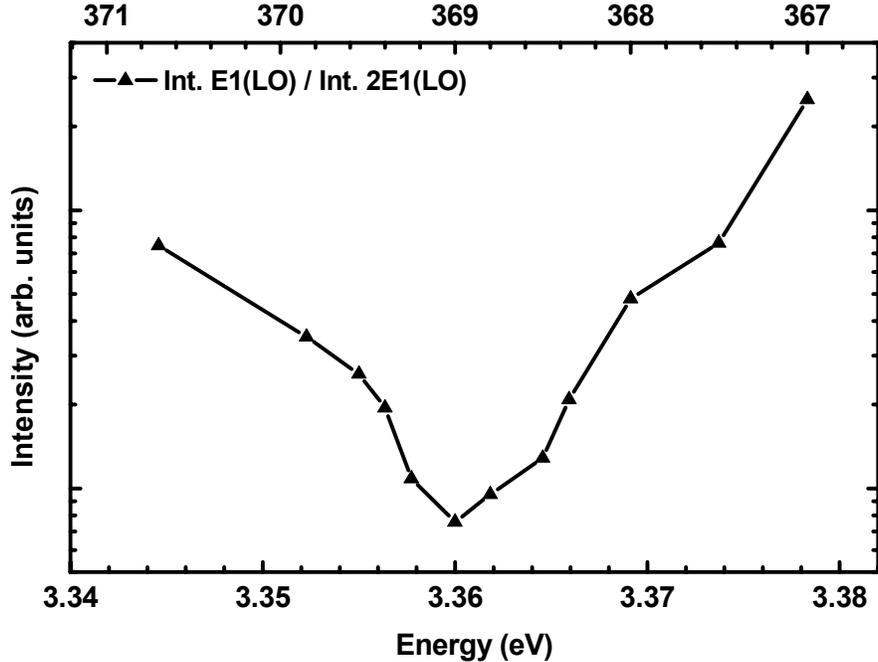
Fig. 9. Intensity ratio of the  $E_1(\text{LO})$  Raman mode divided by the intensity of the  $2E_1(\text{LO})$  Raman peak for different excitation energies (displayed on a logarithmic scale). The solid lines are a guide to the eye only.
