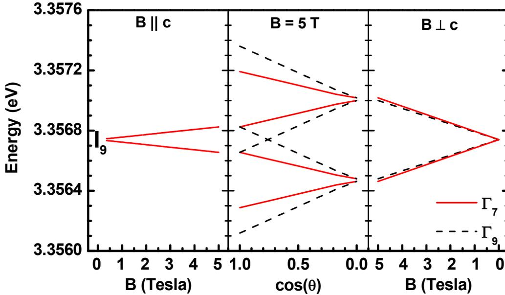
Fig. 4. Calculated Zeeman splitting of the  $I_9$  bound exciton line for holes with  $\Gamma_7$  (solid lines) or  $\Gamma_9$  (dashed lines) symmetry. The splitting as a function of the applied magnetic field is given for  $B \parallel c$  (left) and  $B \perp c$  (right), as well as for arbitrary angles at a constant magnetic field strength of 5 Tesla (middle).
