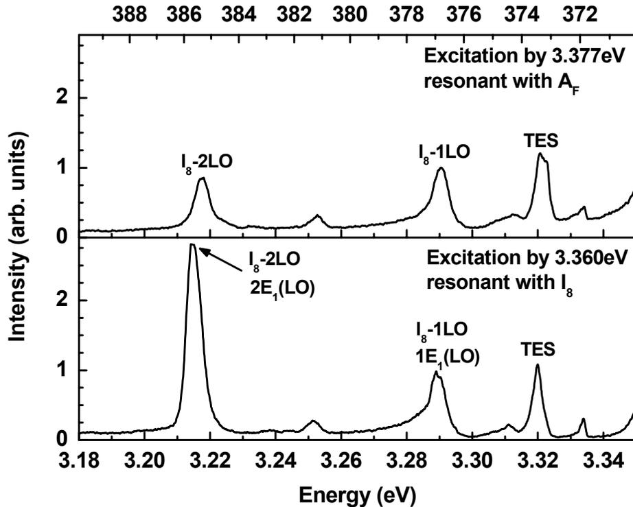
Fig. 8. PL and Raman spectra of CVD grown ZnO at 1.8 Kelvin for two different laser excitation energies. Top graph: Excitation at 3.377eV (in resonance with the  $A_F$  free exciton  $A_F$ ), bottom graph: excitation at 3.360eV (in resonance with the donor bound exciton complex  $I_8$ )
