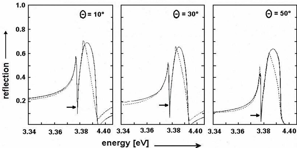
Fig. 2. Reflection spectra at 2 K of high-quality ZnO crystals. The reflectivity is depicted as a function of the excitation energy for angles of 10°, 30° and 50° between the crystal c-axis and the k-vector of the incident light. Solid lines and dashed lines represent the experimental and fitted curves, respectively.
