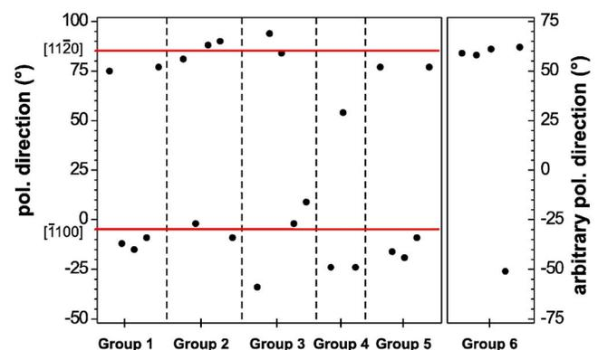
FIG. 3. (Color online) Polarization directions of six different line groups. They scatter around  $[11\bar{2}0]$  and  $[\bar{1}100]$ . Both directions can be found in each line group. For line group no. 6, the alignment of the polarization directions to the crystal axes is unknown. Groups 1–3 correspond to the spectra (a)–(c) in Fig. 2.
