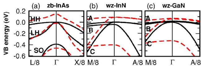
FIG. 4. (Color online) Calculated bulk  $\mathbf{k} \cdot \mathbf{p}$  VB structure of (a) zb-InAs, (b) wz-InN, and (c) wz-GaN; unstrained (black solid lines) and under compressive biaxial strain ( $-3\%$ ) in the basal plane with elastic relaxation along (001) direction (red dashed lines). The splitting between the  $A$  and  $B$  VB at  $\Gamma$  is  $\approx 3$  meV in strained and unstrained InN, and 11 meV (5 meV) in strained (unstrained) GaN.
