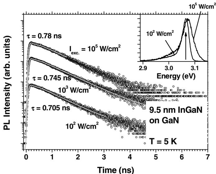
**Figure 2.** Time-resolved PL at 5 K and different excitation densities. Inset: time-integrated PL.
