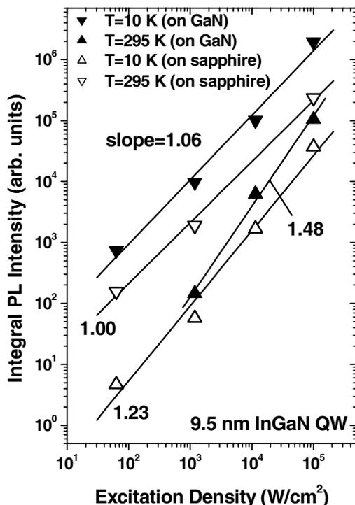
**Figure 4.** Integral PL intensity vs. excitation density at 10 K and room temperature.
