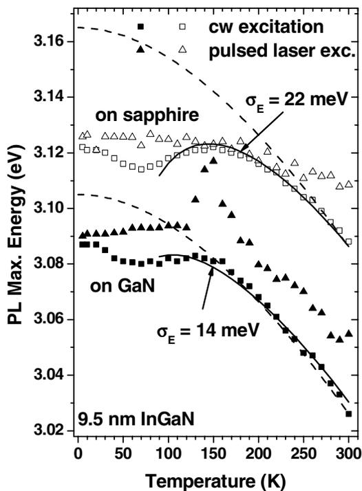
**Figure 1.** Energetic position of the PL maximum vs. temperature at low excitation density (squares) and at high excitation density (triangles). Fit after Refs. 5 and 6 (solid line), band gap behavior of GaN (dashed line).
