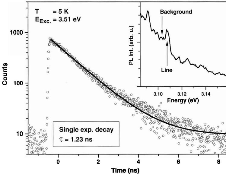
Fig. 5. Time-resolved PL of a single QD emission line (inset), fitted by a monoexponential decay (solid line).
