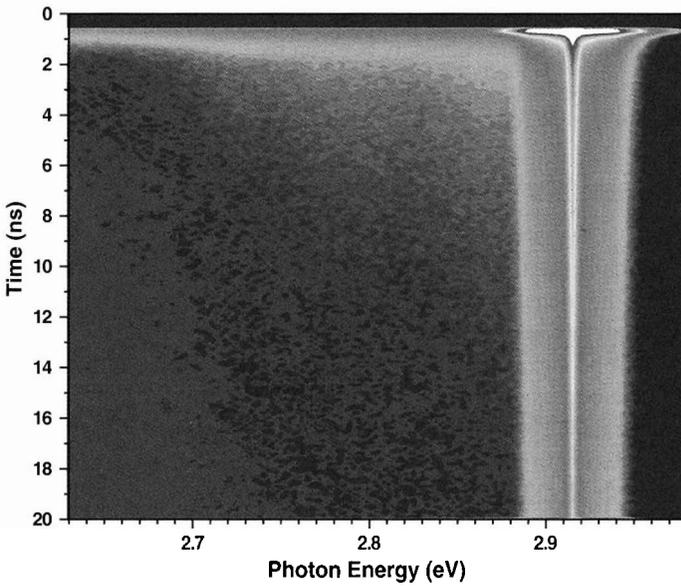
Fig. 2. Time/wavelength plot for resonant excitation (sample A). White spot corresponds to the scattered laser light.
