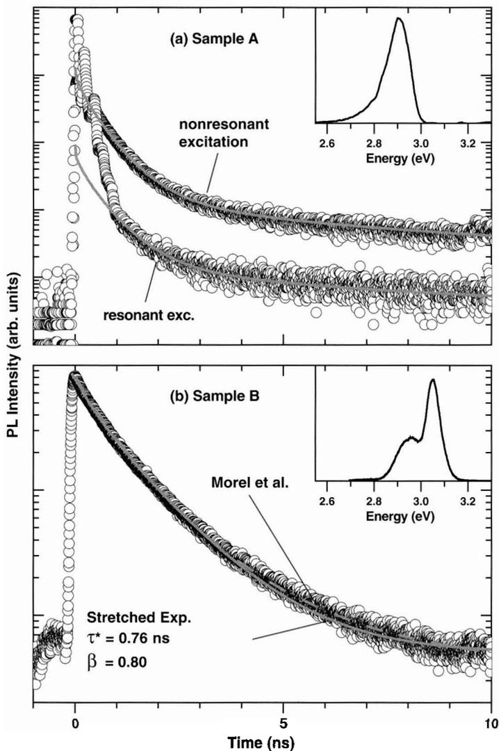
Fig. 1. Time-resolved PL, fits with Eq. (1) (solid lines) and after Morel et al. (dashed line in Fig. 1(b)), inset: time-integrated PL.
