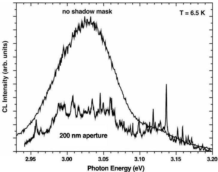
Fig. 3. CL of sample B without shadow mask and through a 200 nm aperture.
