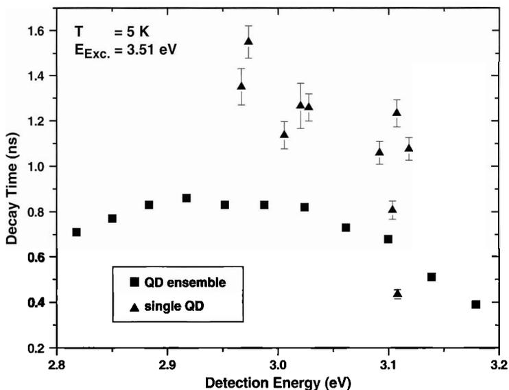
Fig. 6. Spectral dependence of time constants for single QD lines (triangles) and the QD ensemble (squares).
