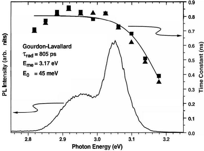
Fig. 4. Time-integrated ensemble PL of sample B, time constant  $\tau_e$  of the  $1/e$ -decay (squares) and the fitting parameter  $\tau^*$  (triangles), fit with Eq. (4) (solid line).
