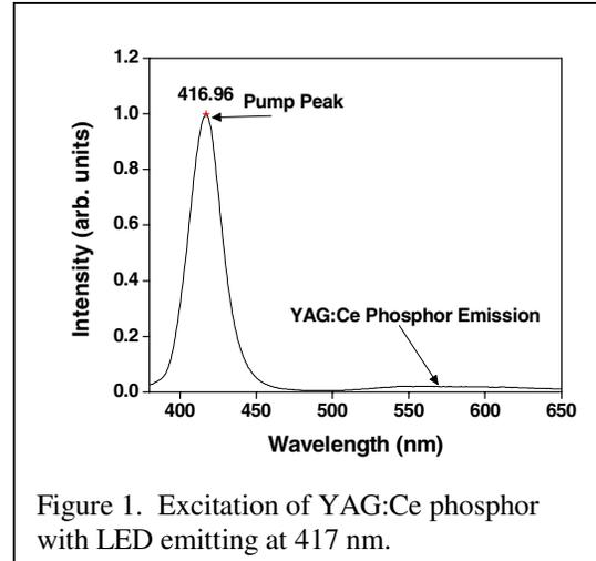
Figure 1. Excitation of YAG:Ce phosphor with LED emitting at 417 nm.
