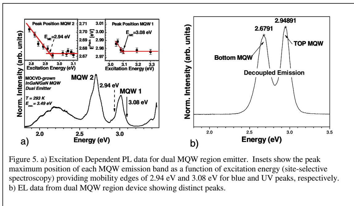
Figure 5. a) Excitation Dependent PL data for dual MQW region emitter. Insets show the peak maximum position of each MQW emission band as a function of excitation energy (site-selective spectroscopy) providing mobility edges of 2.94 eV and 3.08 eV for blue and UV peaks, respectively. b) EL data from dual MQW region device showing distinct peaks.
