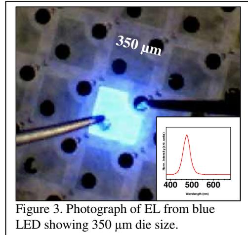
Figure 3. Photograph of EL from blue LED showing 350 μm die size.
