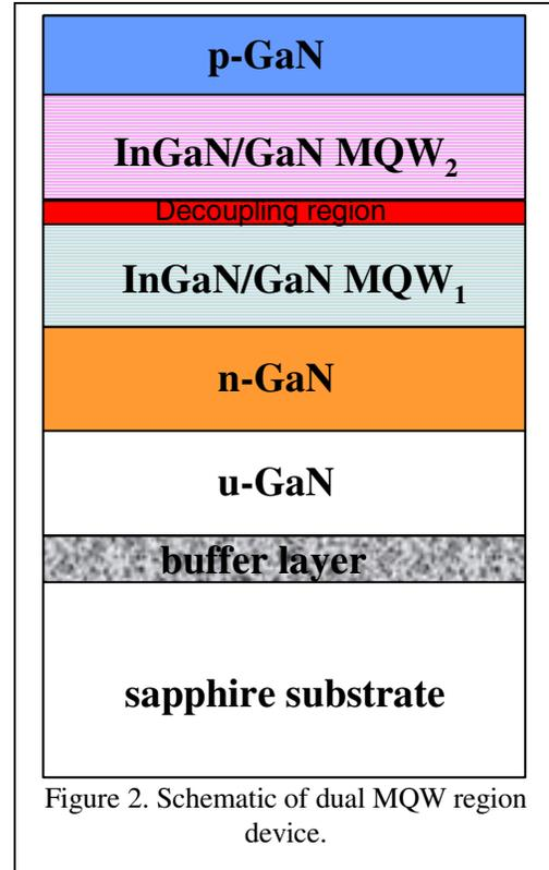
Figure 2. Schematic of dual MQW region device.
