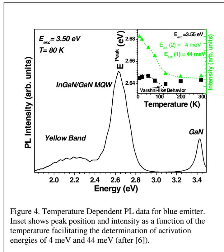
Figure 4. Temperature Dependent PL data for blue emitter. Inset shows peak position and intensity as a function of the temperature facilitating the determination of activation energies of 4 meV and 44 meV (after [6]).
