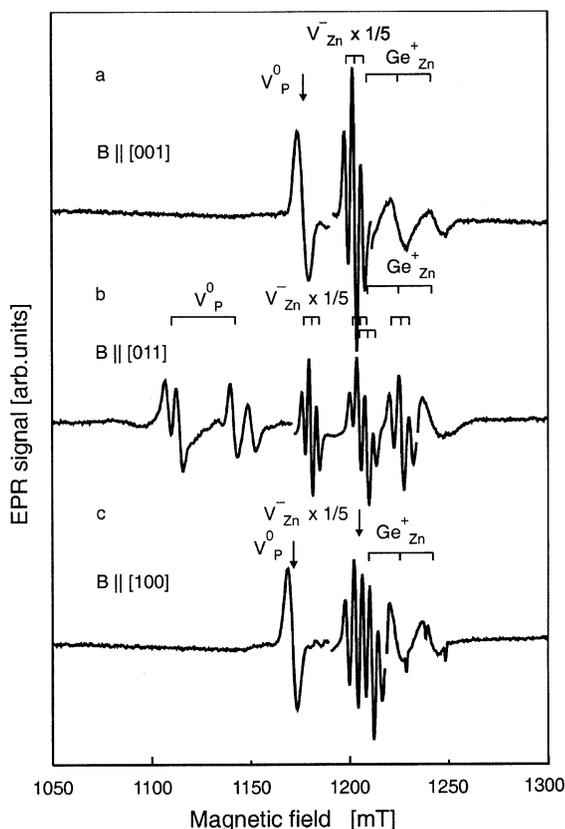
Fig. 1. EPR and photo-EPR spectra of the negatively charged zinc vacancy ( $V_{Zn}^-$ ), the neutral donor ( $V_P^0$ ), and the anti-site centre  $Ge_{Zn}^+$  in as-grown and annealed HGF  $ZnGeP_2$  in the Q-band ( $\nu = 34.2 \text{ GHz}$ ,  $T = 10 \text{ K}$ ) with the magnetic field  $B$  parallel to the crystallographic main directions [001], [011] and [100].
