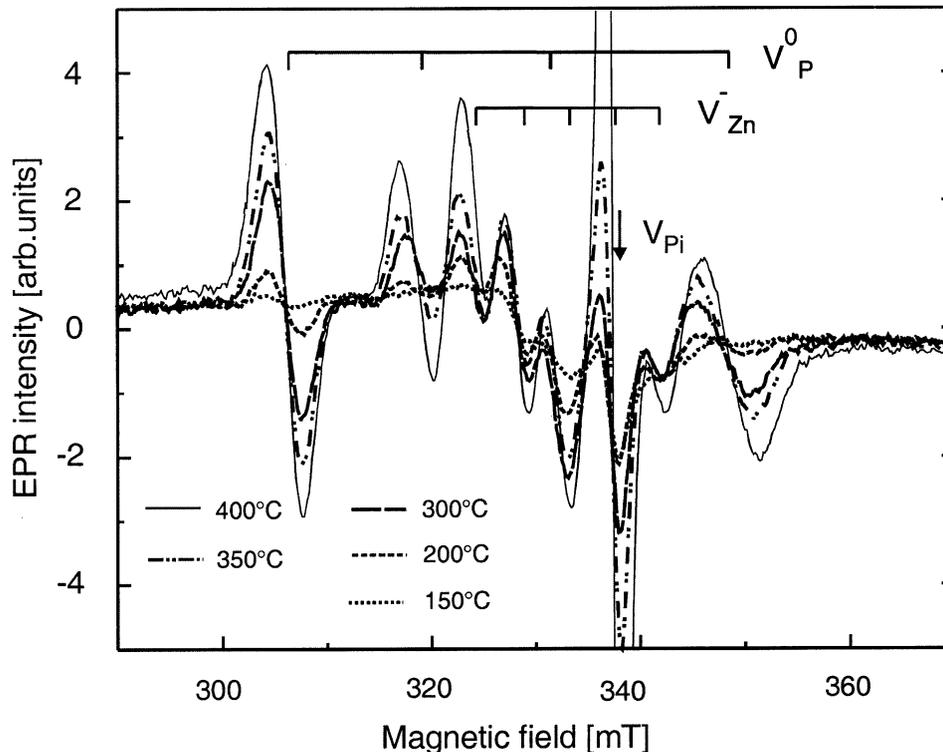
Fig. 4. Dependence of the EPR signal intensities observed under the same conditions as in Fig. 3b, but illuminated with the light of a halogen lamp cut off to  $\lambda > 1.06 \mu$  with a silicon edge filter. The increase of the EPR signal intensities related to the  $V_P^0$ ,  $V_{Zn}^-$ , and isotropic line at  $g = 2.0026$  corresponds to the increase of the annealing temperature similar to Fig. 3b. The intensity of the isotropic line is not affected by the illumination.
