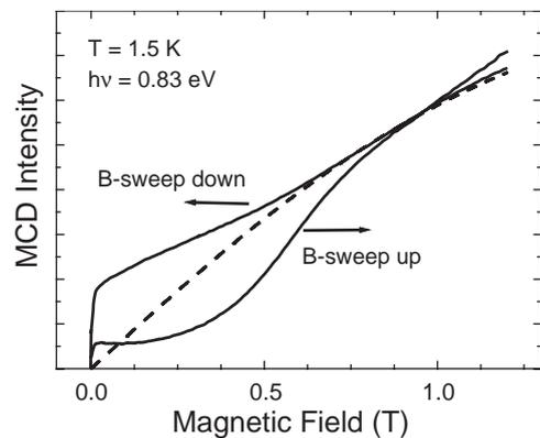
Fig. 4. Magnetic field dependence of the Zn-vacancy-related magnetic circular dichroism for sweeping the magnetic field ( $B$ ) down and up. The dashed line indicates the expected behavior (Brillouin function) for this  $S = \frac{1}{2}$  system.
