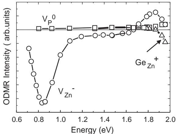
Fig. 3. Spectral dependence of the ODMR signals of the three dominant native defects observed in  $\text{ZnGeP}_2$ .
