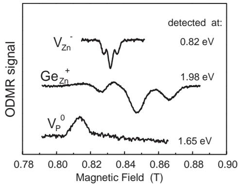
Fig. 2. Optically detected magnetic resonance spectra observed in  $\text{ZnGeP}_2$ . The optical detection energy is given in the figure. (24 GHz, crystal orientation: magnetic field parallel to  $c$ -axis).
