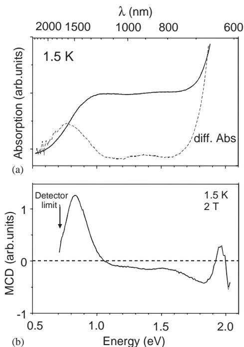
Fig. 1. Absorption spectrum (a) and (b) magnetic circular dichroism (MCD) of  $ZnGeP_2$  crystals grown by the HGF technique. The dashed line in (a) shows the first derivative of the absorption spectrum.
