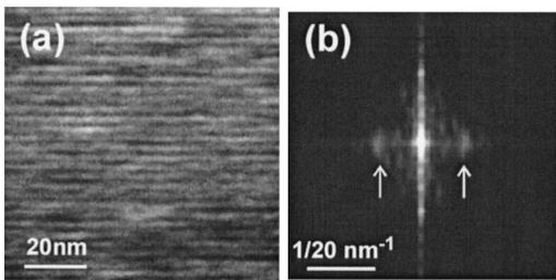
FIG. 1. (a) 004 bright-field TEM image of the structure. (b) 2D Fourier transformation of the TEM image.
