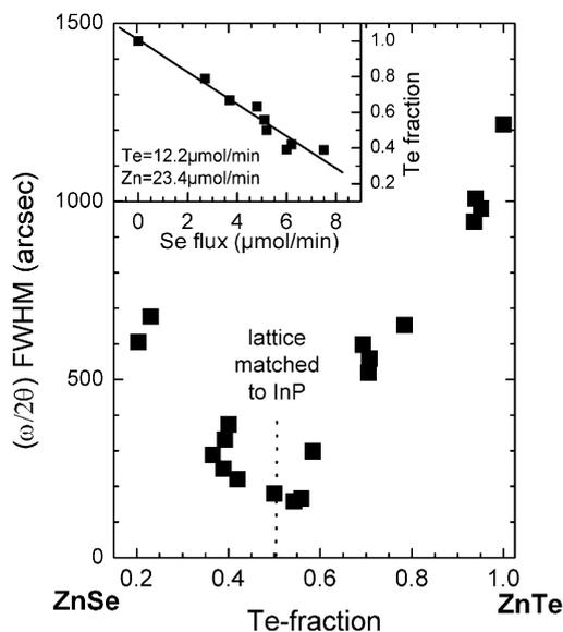
Fig. 1. Dependence of Te incorporation into ZnSe<sub>1-x</sub>Te<sub>x</sub> layers on the gas phase composition (inset) and influence of the composition on the  $\omega/2\theta$  X-ray reflection FWHM.
