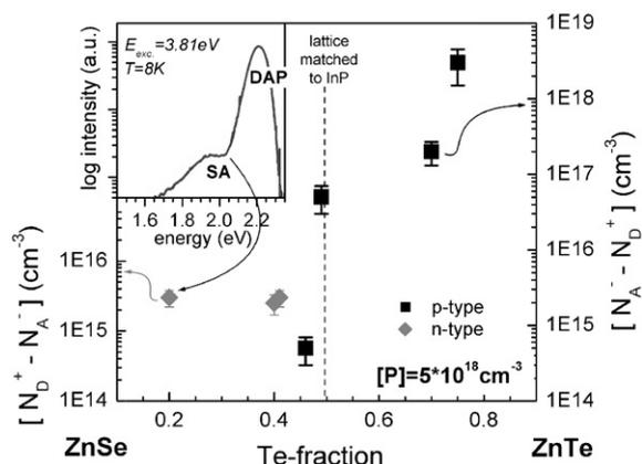
Fig. 5. Free carrier concentration in  $\text{ZnSe}_{1-x}\text{Te}_x$  as a function of the Te fraction; p-type conductivity occurs for a fraction above 0.46. The PL spectrum of  $\text{ZnSe}_{0.8}\text{Te}_{0.2}$  shows the DAP and the SA emission (inset).
