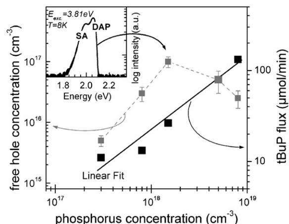
Fig. 4. Dependence of the phosphorus incorporation into ZnSe<sub>0.5</sub>Te<sub>0.5</sub> on the tertiarybutylphosphine flux in the gas phase (right) and free hole concentration as a function of the phosphorus concentration (left). The PL spectrum of ZnSe<sub>0.5</sub>Te<sub>0.5</sub>:P (sample (d)) shows the DAP and the SA emission (inset).
