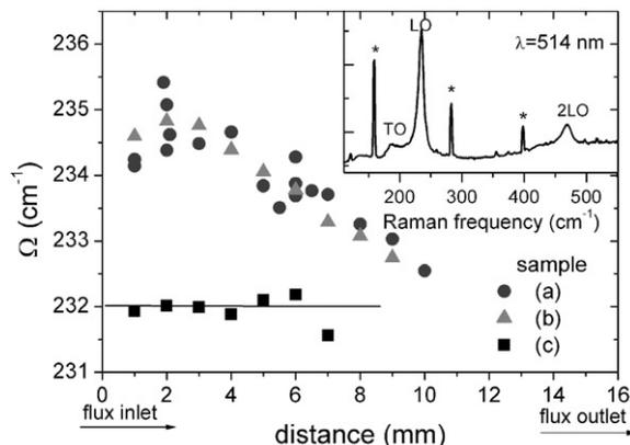
Fig. 3. Raman microanalysis of ZnSeTe layers with differently thick ZnCdSe buffers along the direction inlet to outlet of the precursor flux during growth (for detailed discussion see text). Sample (c) shows no systematic lateral dependency of the Raman frequency. Inset: Characteristic Raman spectrum of sample (a) excited at 514 nm. Peaks marked with stars are emission lines from an Ar lamp used for calibration.
