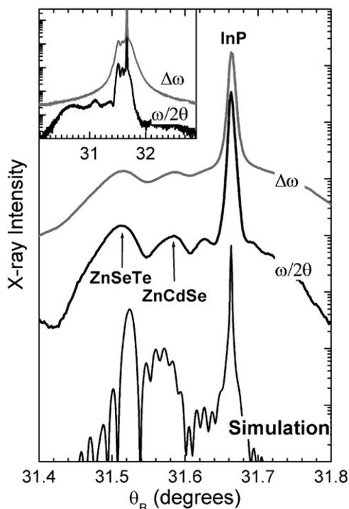
Fig. 2. Comparison between  $\omega/2\theta$  and  $\Delta\omega$  X-ray spectra for an almost lattice matched alloy of  $\text{ZnSe}_{0.47}\text{Te}_{0.53}$  on a ZnCdSe buffer on InP. The broadening of the  $\Delta\omega$  curve shows the mosaic in the layer (for detailed discussion see text). The extended  $\omega/2\theta$  scan reveals compositional fluctuations (inset).
