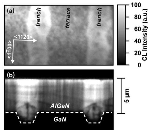
FIG. 5. Modulation of AlGaIn quantum efficiency with pattern periodicity: CL intensity images integrating the AlGaIn emission (300–340 nm) of the (a) as-grown sample surface, and (b) the corresponding cross section perpendicular to the trench direction.
