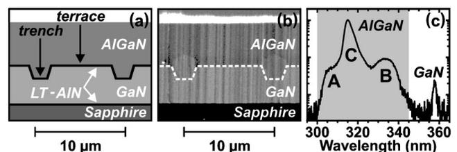
FIG. 1. (a) Schematic sample structure, (b) cross-sectional SEM image perpendicular to the trench direction, and (c) CL spectrum averaging the emission of the area shown in (b).
