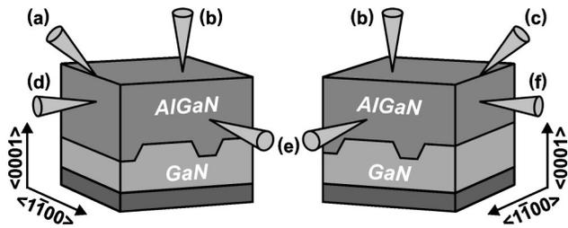
FIG. 2. Schematic illustration of the CL scan orientations used for the set of CL wavelength images in Figs. 3(a)–3(f).
