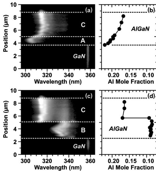
FIG. 4. Evolution of CL emission and aluminum content along  $\langle 0001 \rangle$ : (a) and (b) above terrace; (c) and (d) above trench, respectively. [In the CL linescans Figs. 3(a) and 3(c) bright contrast means high CL intensity.]
