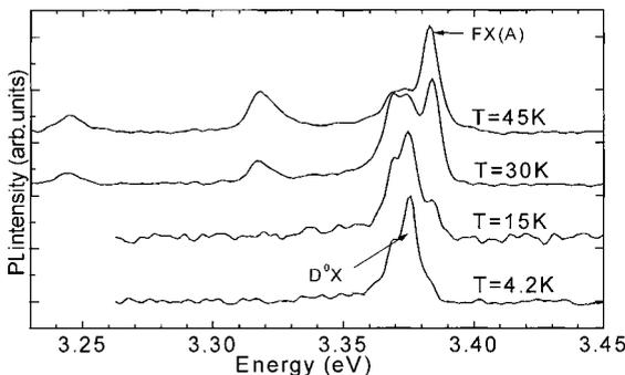
Fig. 3. Photoluminescence spectra measured with low resolution set-up for epitaxial ZnO at 4.2, 15, 30 and 45 K. The free and D<sup>0</sup>X exciton transitions are indicated by arrows
