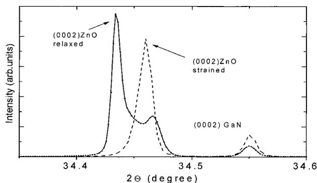
Fig. 1. X-ray diffraction of ZnO epilayers on (0002) GaN templates for a 1 μm thick film (dashed line) and for a film thickness of 15 μm (solid line)
