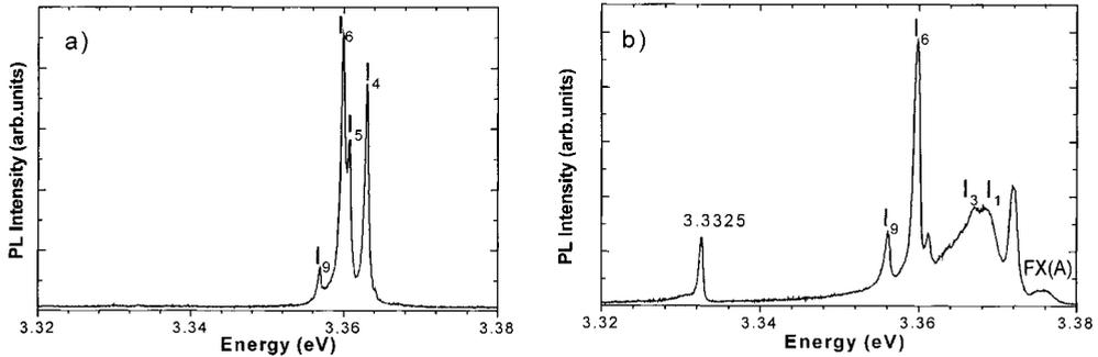
Fig. 2. Photoluminescence spectra (4.2 K) of a) bulk ZnO single crystal and b) ZnO epitaxial film (thickness 1 μm), for details see text
