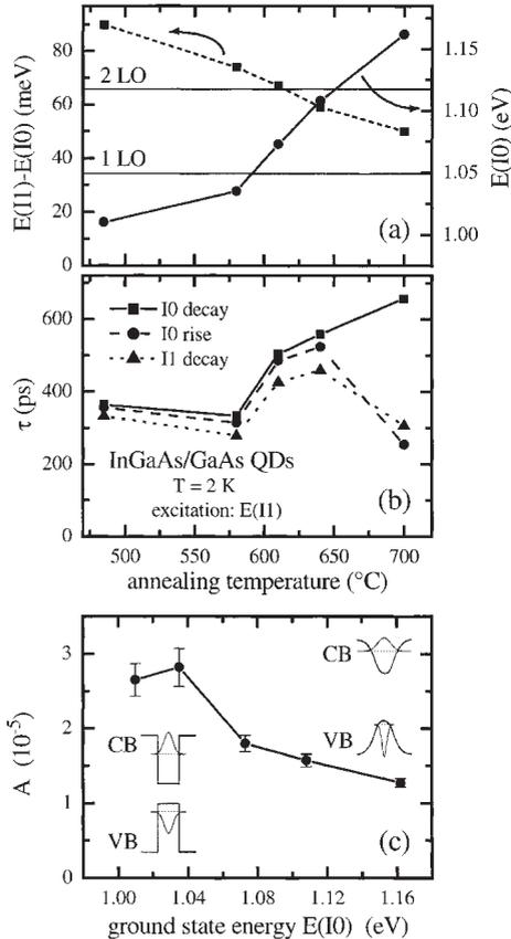
Fig. 3. Properties of ex-situ annealed InGaAs/GaAs QDs: a) the ground state transition energy and the I1/I0 splitting derived from high-density PL spectra; b) the rise and decay times of I0 and I1 upon resonant excitation of I1; c) the dimensionless factor  $A = (P_{\text{CV}}/\hbar c)^2 I$  being proportional to the oscillator strength. The insets illustrate schematically the effect of the annealing-induced smoothing of the confining potential on the electron and hole localization
