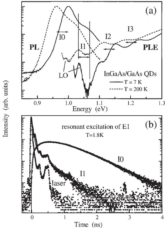
Fig. 2. a) PL and PLE spectra of a typical InGaAs QD sample. The solid and dotted lines represent spectra recorded at 7 and 200 K, respectively. b) Transients of the ground (I0) and first excited (I1) state PL upon resonant excitation of excitons in the first excited state
