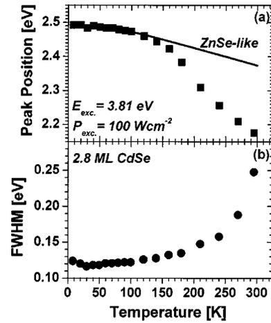
FIG. 2. PL emission maximum (a) and half width (FWHM) of the emission band (b) as a function of the temperature between 2 and 300 K. The solid line shows the temperature dependence of the ZnSe band gap.
