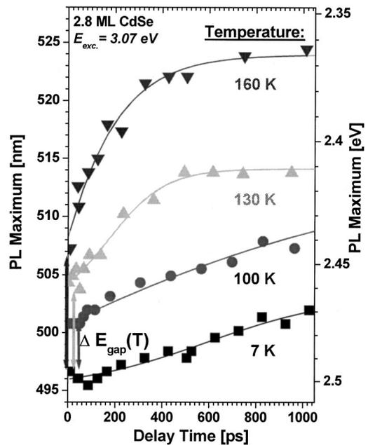
FIG. 3. PL maximum as a function of the delay time. The data were recorded at 7, 100, 130, and 160 K, respectively. The least-square root fits are introduced to guide the eye. The vertical arrows near  $t=0$  ps mark the redshift due to the temperature dependence of the band gap at the corresponding temperatures.
