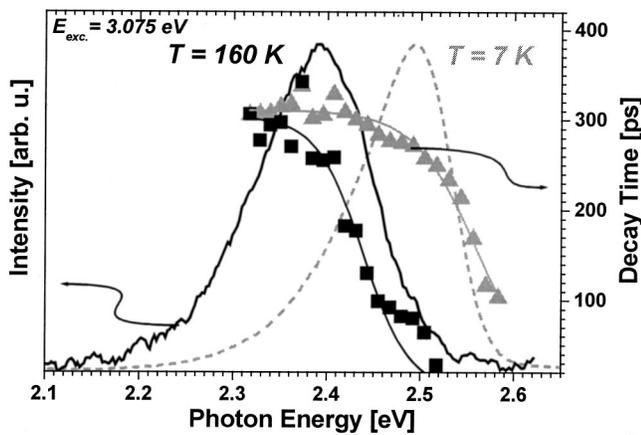
FIG. 4. Time-integrated photoluminescence and decay constants as a function of the detection energy recorded at 7 and 160 K. Equation (1) was applied to fit the decay-time dependence.
