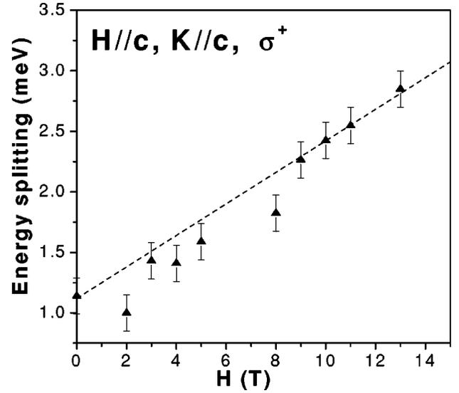
FIG. 7. Magnetic field dependence of the splitting between uppermost and lowest peaks of the surface emission from the  $n=1$  state of the  $A$  exciton measured with  $\sigma^+$  polarization for magnetic field and wave vector parallel to the hexagonal axis ( $\mathbf{K}\parallel c$ ,  $\mathbf{H}\parallel c$ ). Sample I.
