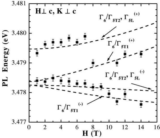
FIG. 6. Magnetic field dependence of the energy peaks of the edge emission from the  $n=1$  state of the  $A$  exciton for magnetic field and wave vector perpendicular to hexagonal axis ( $\mathbf{K}\perp c$ ,  $\mathbf{H}\perp c$ ). Sample I.
