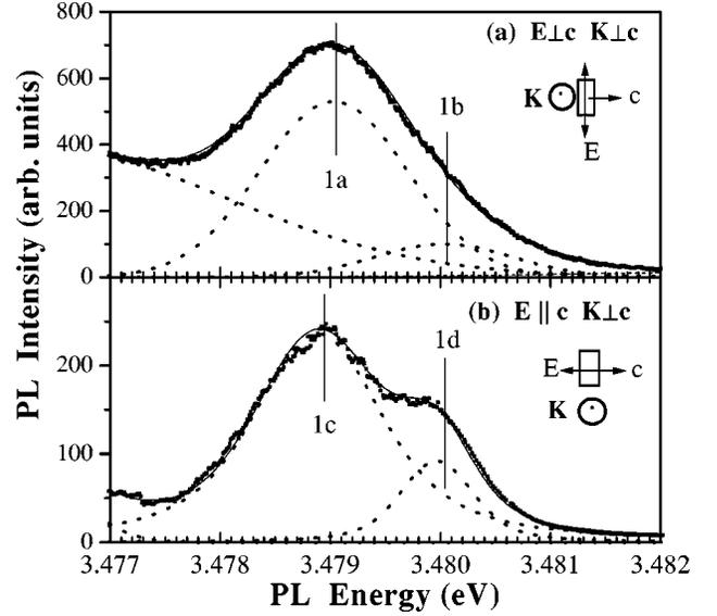
FIG. 4. Linearly polarized edge emission from the  $n=1$  state of the  $A$  exciton: (a)  $\mathbf{E} \perp c$  and (b)  $\mathbf{E} \parallel c$ . Symbols represent experimental data, dashed lines fitted individual peaks; the solid line is the fit to the measured spectrum. Sample I.
