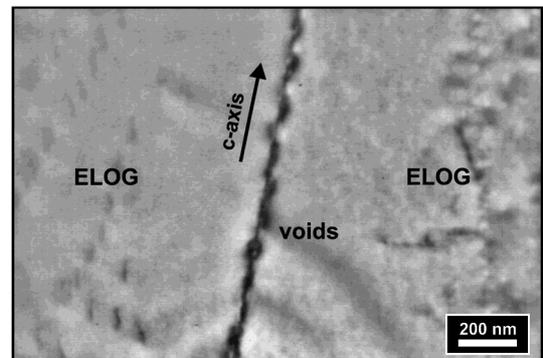
Fig. 1. TEM image of the voids observed in the coalescence region of the  $\langle 11\bar{2}0 \rangle$  sample of GaN ELOG. A similar image is observed for the  $\langle 1\bar{1}00 \rangle$  sample.
