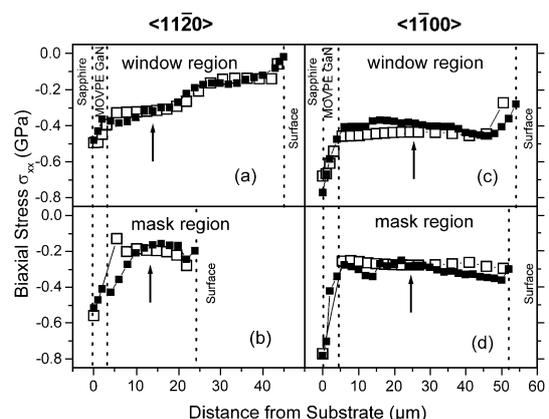
Fig. 3. Comparison of theoretical (white boxes) and experimentally derived (black boxes) biaxial stresses  $\sigma_{xx}$  along the window loci WW’ and mask loci MM’ in the samples. The arrows indicate the positions of the cross sectional area ABCD of Figs. 2 and 4.
