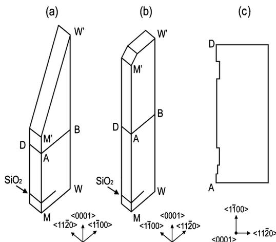
Fig. 2. (a) FEM unit cell of the  $\langle 11\bar{2}0 \rangle$  sample; (b) FEM unit cell of the  $\langle 1\bar{1}00 \rangle$  sample; (c) schematic form of the voids used in the FEM.
