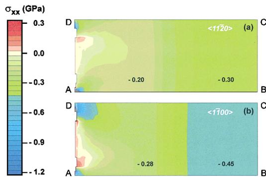
Fig. 4. Theoretical biaxial stress  $\sigma_{xx}$  on the cross-sectional surface ABCD in the samples.
