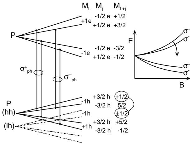
Fig. 8. Level scheme indicating allowed optical transitions between the first excited states of the dots. As illustrated in the inset, coupling between heavy and light-hole states of same symmetry (circled ones) leads to a reduction of the magnetic-field splitting of the emission lines in  $\sigma^+$  polarization.
