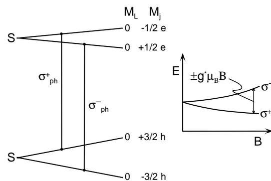
Fig. 6. Level scheme indicating allowed optical transitions between electron and hole ground states of the quantum dots. States are labelled according to their  $z$  component  $M_L$  of the envelope angular momentum and  $M_j$  of the atomic one. The inset schematically represents the energy splitting of the corresponding emission with  $\sigma^\pm$  polarization in a magnetic field.
