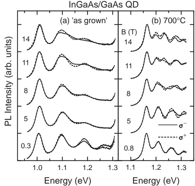
Fig. 2. Photoluminescence spectra of an InGaAs/GaAs quantum dot structure (a) as grown and (b) annealed at 700°C measured using high excitation powers of 5 kW/cm<sup>2</sup> for different magnetic fields and at 2 K. The solid (dashed) lines correspond to  $\sigma^-$  ( $\sigma^+$ ) circular polarization.
