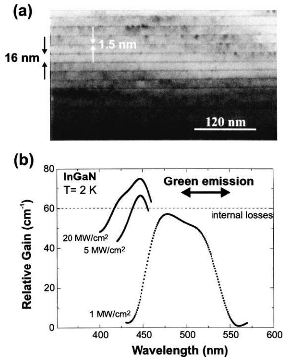
Fig. 8. (a) Transmission electron microscopy image of multiple InGaN–GaN insertions in a GaN matrix emitting in the green spectral range. The average thickness of the InGaN insertions is only about two monolayers. (b) Gain spectra measured in the same structure. Note the significant relative gain in the green spectral range.
