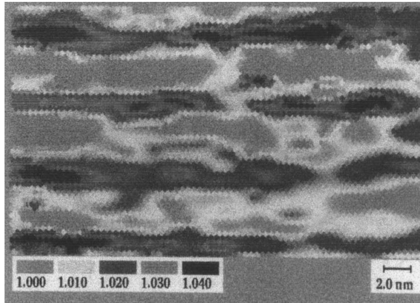
Fig. 1. The color-coded map of the local lattice parameter (LLP) in growth direction digitally processed from a HRTEM image of a stacked submonolayer-CdSe/ZnMgSSe structure with 3 nm spacer thickness.
