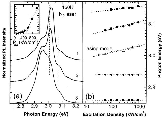
Fig. 6. (a) PL spectra at different excitation densities 1, 1 MW/cm<sup>2</sup>; 2, 0.59 MW/cm<sup>2</sup>; 3, 0.16 MW/cm<sup>2</sup> (PL intensity vs. excitation density is shown in the inset). (b) Cavity mode energies vs. excitation density.
