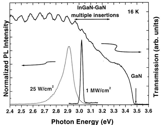
Fig. 5. Low-temperature PL spectra at low and high excitation densities and optical transmission spectrum of the structure. PL intensity vs. excitation density is shown in the inset.
