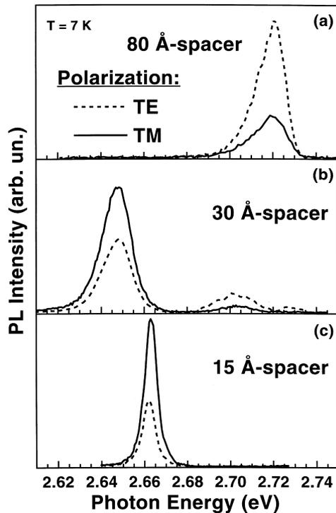
Fig. 3. Linearly polarized photoluminescence (PL) of structures with 80 Å (a), 30 Å (b) and 15 Å (c) spacers measured in edge geometry. The polarization changes from mostly TE for uncoupled islands (80 Å spacers) to mostly TM (accompanied by a red shift) for vertically coupled islands (15 Å spacers). The 30 Å spacer sample shows emission from both types of islands.
