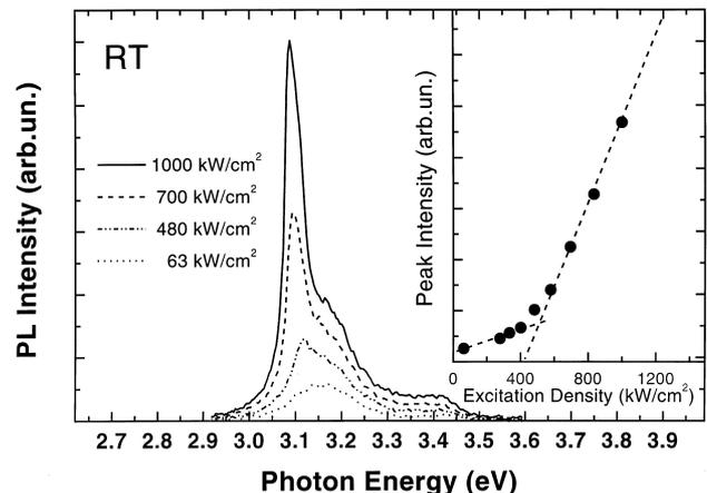
Fig. 7. Room-temperature photoluminescence (PL) spectra of the VCSEL structure at different excitation densities (solid line, 1000 kW/cm<sup>2</sup>; dashed line, 700 kW/cm<sup>2</sup>; short dashed line, 480 kW/cm<sup>2</sup>; dotted line, 63 kW/cm<sup>2</sup>). Inset shows dependence of the peak PL intensity on excitation density.
