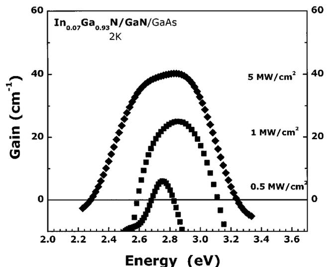
FIG. 3. Gain measurements at various excitation densities of an In<sub>0.07</sub>Ga<sub>0.93</sub>N sample.
