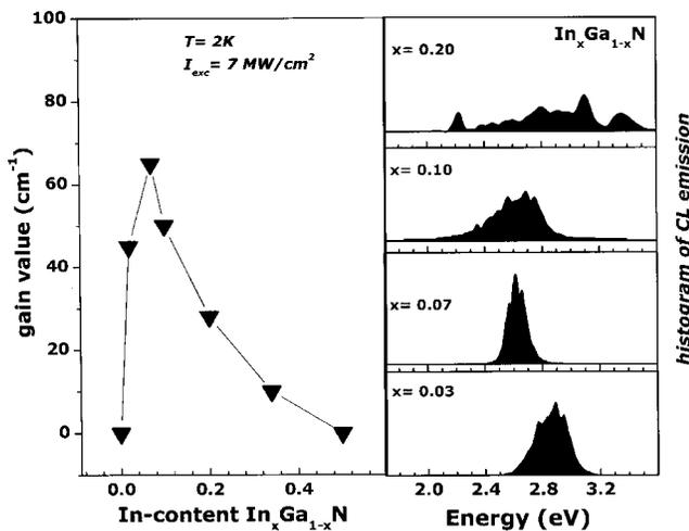
FIG. 4. (right hand side) Comparison of the peak gain values at an excitation density of  $7 \text{ MW/cm}^2$  for  $c\text{-InGaN}$  samples with different In content. (left hand side) Results of the cathodoluminescence measurements. Displayed are the histograms of the CLWI for  $c\text{-InGaN}$  samples with varying In content.
