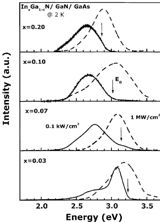
FIG. 1. Comparison of low-excitation PL (full curves) and the high-excitation edge emission (dotted curves) of *c*-InGaN samples with varying In content. The values of the band gap, determined by reflectivity, are indicated by arrows.
