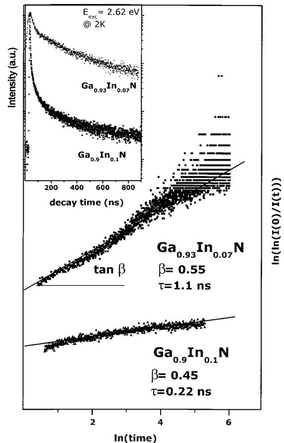
FIG. 2. The transients of the two samples with In contents of 7% and 10% plotted according to the model of stretched exponentials. The values for  $\tau$  and  $\beta$  can be determined by plotting  $\ln\{\ln[I(0)/I(t)]\}$  vs  $\ln(t)$ . (Inset) Luminescence decay of the two *c*-InGaN samples.
