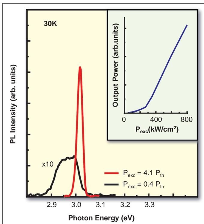
**Figure 2.** Low temperature photoluminescence spectra below and above threshold for a structure with twelve InGaN insertions in a GaN matrix, grown without both top and bottom DBRs. ( $P_{exc}$  = excitation density,  $P_{th}$  = threshold density). Inset: Output power versus excitation density for the same structure.
