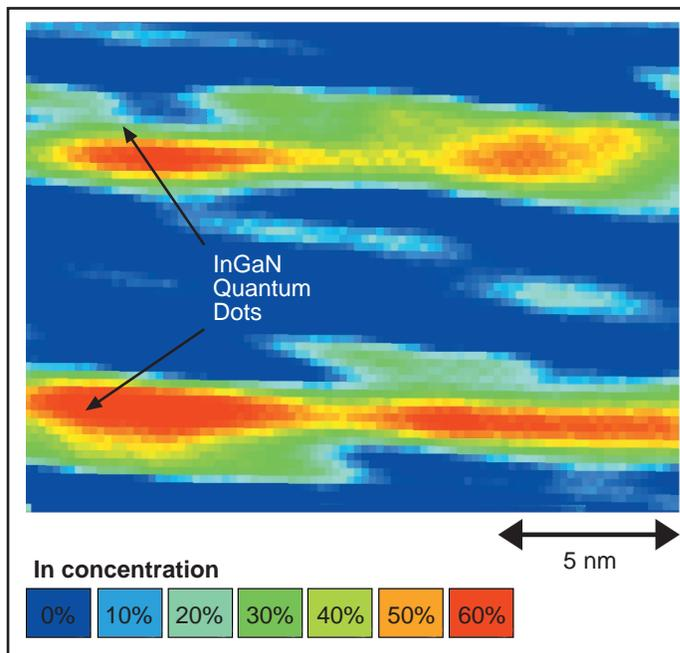
**Figure 1.** Color-coded map of indium distribution in structure with multiple ultra-thin InGaIn insertions evaluated using cross-section high-resolution transmission electron microscopy and DALI image-processing (courtesy of Laboratorium für Elektronmikroskopie der Universität Karlsruhe). The active region was formed by temperature cycling during InGaIn layer growth (average In content ~10%).
