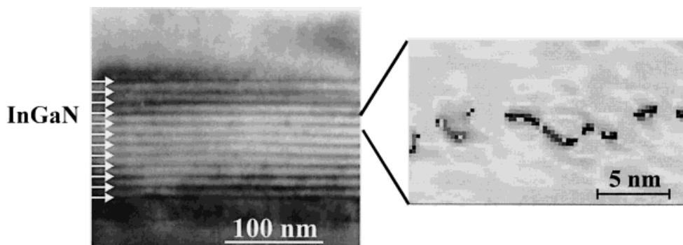
Fig. 1. a) Cross-sectional TEM image for the “violet” structure and b) DALI processed image of one InGaIn insertion (black color represents higher In content)
