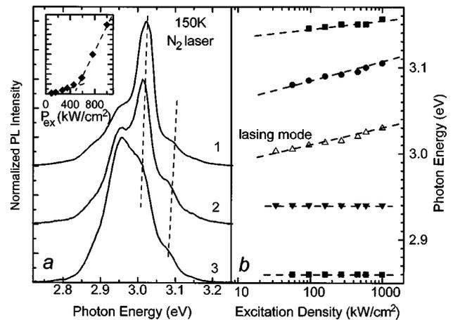
FIG. 3. PL spectra at different excitation densities (a) 1—1 MW/cm<sup>2</sup>, 2—0.59 MW/cm<sup>2</sup>, 3—0.16 MW/cm<sup>2</sup> (PL intensity vs excitation density is shown in the insert), and cavity mode energies vs excitation density (b).
