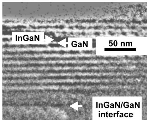
FIG. 1. Cross-section TEM image of the structure. The GaN/InGaN interface and one of the InGaN insertions are marked by arrows.
