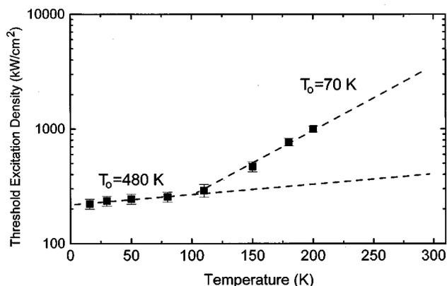
FIG. 4. Temperature dependence of the threshold excitation density for lasing in the direction perpendicular to the surface.
