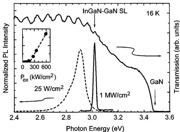
FIG. 2. Low-temperature PL spectra at low and high excitation densities and optical transmission spectrum of the structure. PL intensity vs excitation density is shown in the insert.
