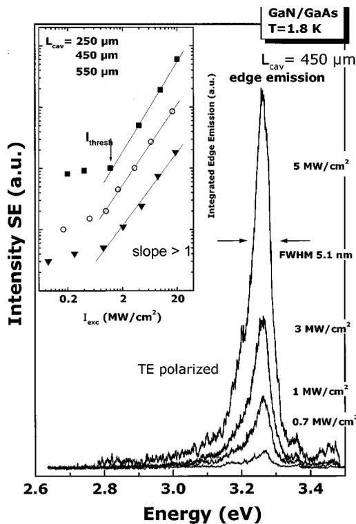
FIG. 1. Polarized edge emission from a cleaved *c*-GaN/GaAs sample with a 450  $\mu\text{m}$  cavity at different excitation densities at 1.8 K. (a) (inset of Fig. 1) Summarized data of intensity dependent edge emission spectra from cleaved cavity samples (integrated edge emission versus excitation density).
