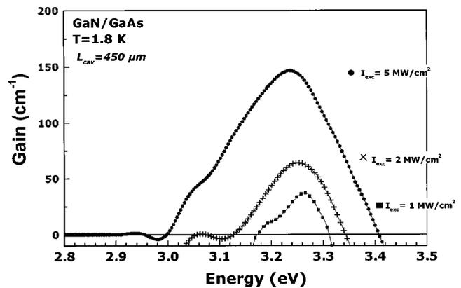
FIG. 3. Gain spectra of *c*-GaN (450  $\mu\text{m}$  cavity) for various excitation densities up to 5  $\text{MW}/\text{cm}^2$  at 1.8 K.
