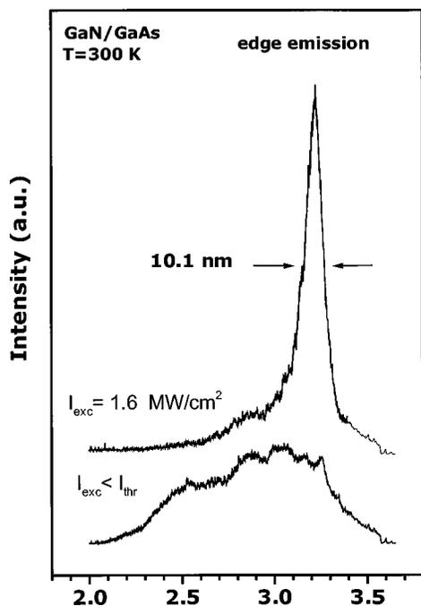
FIG. 2. Edge emission at room temperature from a *c*-GaN sample with a cavity length of 450  $\mu\text{m}$ , the upper spectrum shows the stimulated emission above 1.6  $\text{MW}/\text{cm}^2$ , the lower spectrum is the broad, unstructured emission below threshold.
