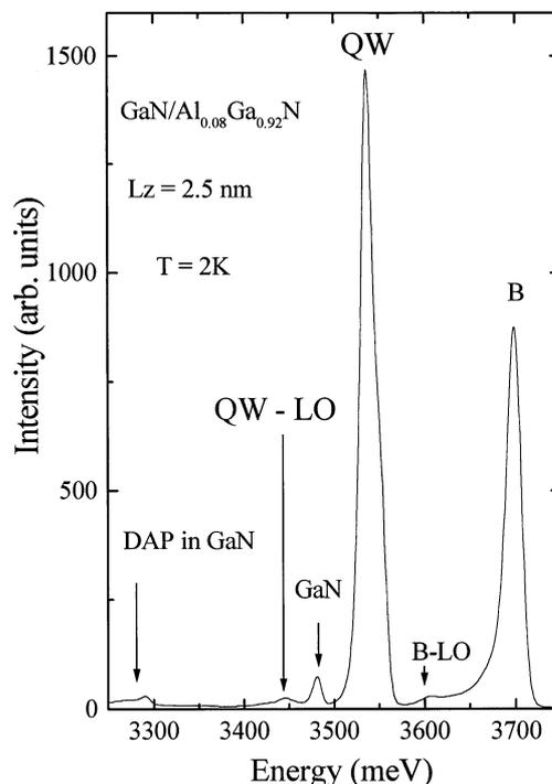
Fig. 1. 2K photoluminescence spectrum of the GaN–AlGaN MQW.
