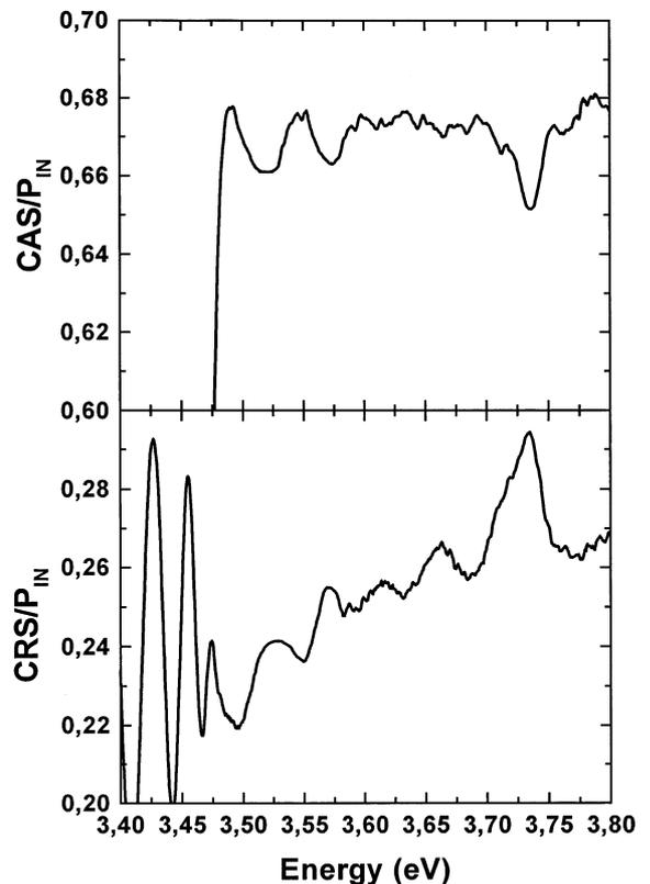
Fig. 3. High resolution plot of the CAS and the CRS spectra.
