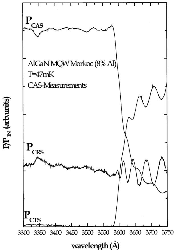
Fig. 2. Typical microcalorimetry spectra taken at 47 mK. Spectra correspond to micro calorimetric absorption, reflection, and transmission, respectively.
