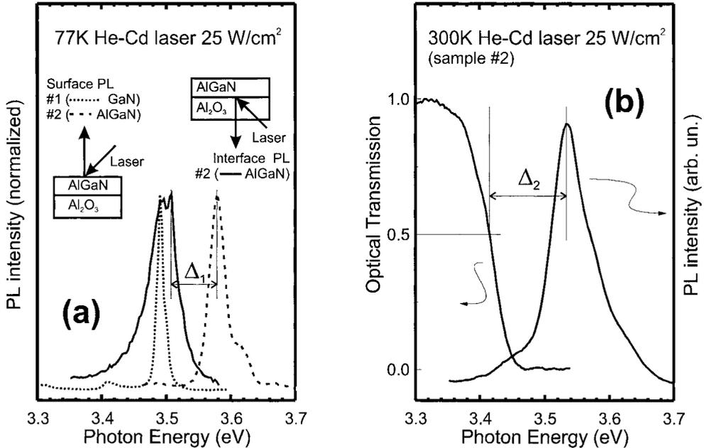
Fig. 1. a) Low temperature PL spectra of the structure grown with constant TMG flow (#2) recorded from near-surface and near-interface regions. b) Room temperature optical transmission and surface PL spectra for the structure grown at constant TMG flow (#2)
