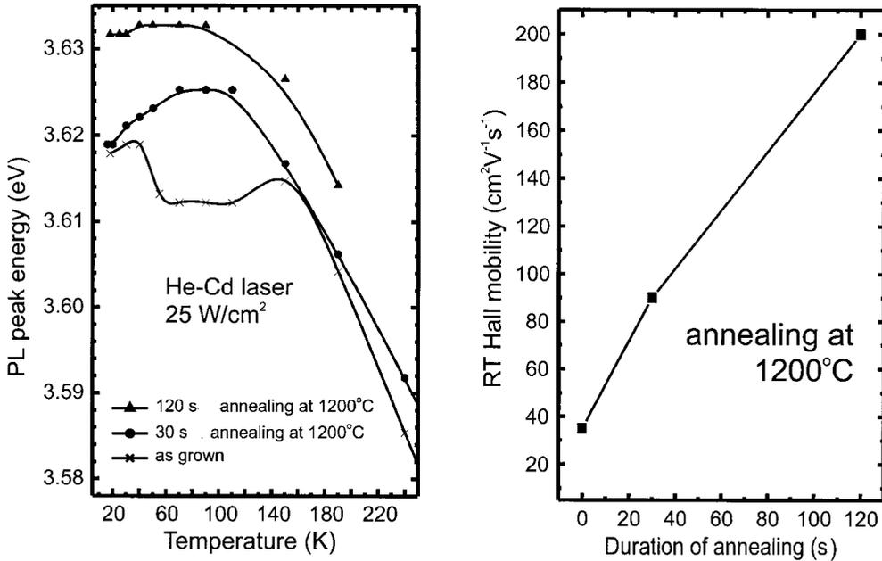
Fig. 3. a) Near-band-edge PL peak energy versus temperature recorded for the as-grown and annealed AlGaIn epilayer. b) Dependence of room temperature electron Hall mobility in the AlGaIn epilayer on duration of rapid thermal annealing
