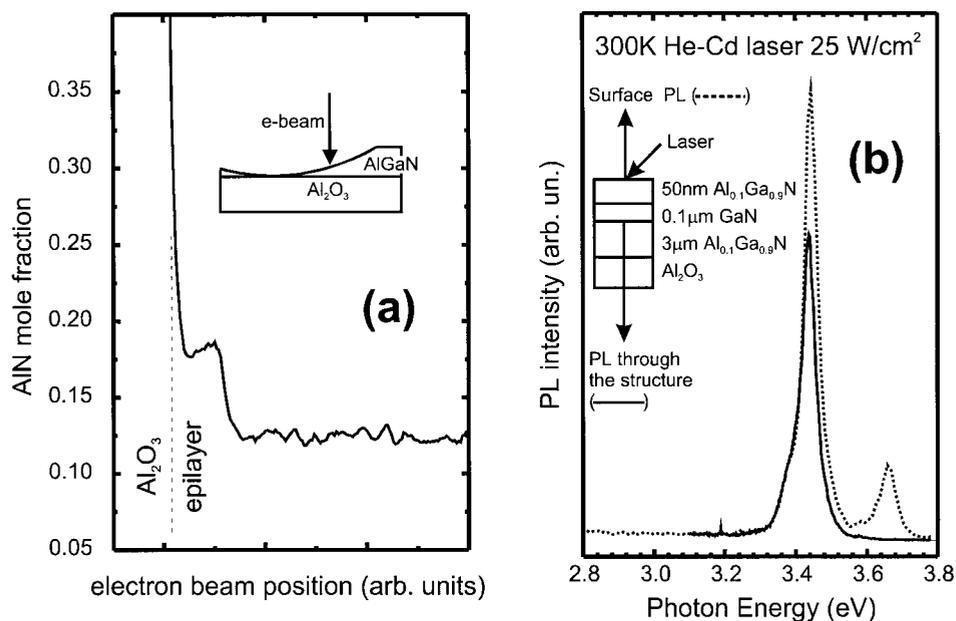
Fig. 2. a) Al distribution for the structure grown with varied TMG flow (#4) and AlN-coated susceptor. b) PL spectra for AlGaN/GaN/AlGaN DHS recorded in two different geometries
