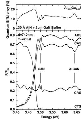
**Figure 3.** CAS/CTS/CRS/ABS-spectrum of a AlGaIn epilayer (6 % Al); the calculated quantum efficiency is shown in the upper part.
