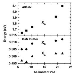
**Figure 4.** Dependence of the absorption energies of the  $X_A$ -resonance in AlGaN on the Al-content (upper part); in the lower part the  $X_A$ - and the  $X_B$ -resonance energies of the GaN buffer layer are shown.
