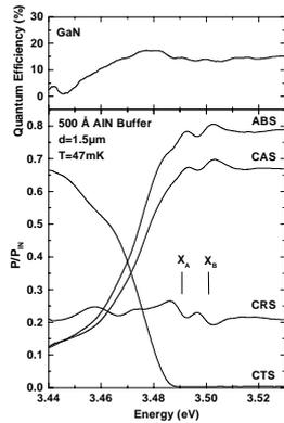
**Figure 1.** CAS/CTS/CRS/ABS-spectrum of a GaN epilayer; the calculated quantum efficiency is shown in the upper part.
