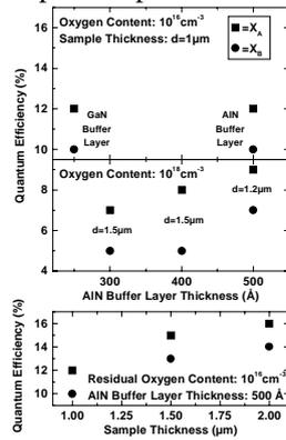
**Figure 2.** Dependence of the qe of the  $X_A$  and  $X_B$  resonances in GaN on the buffer layer thickness for different oxygen contents ( $\uparrow 10^{16} \text{cm}^{-3}$   $\downarrow 10^{18} \text{cm}^{-3}$ ) and on the sample thickness for an oxygen content of  $10^{16} \text{cm}^{-3}$ .
