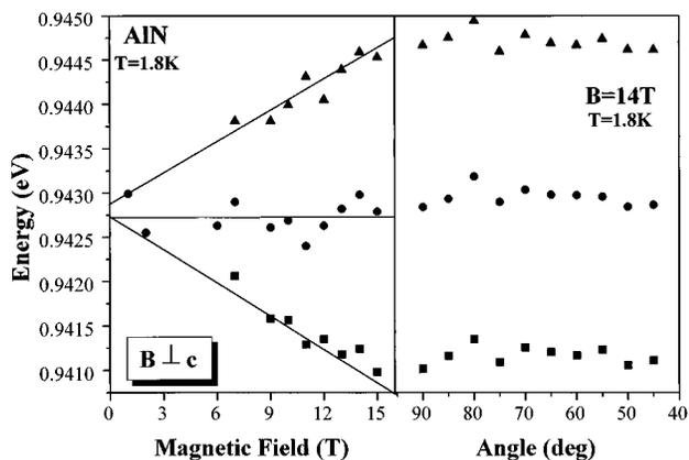
FIG. 2. Zeeman behavior of the 0.943 eV ZPL for  $B \perp c$  (left) and angular dependence at  $B=14$  T (right). The zero-field splitting of  $120 \pm 30 \mu\text{eV}$  together with the  $g$  value of  $1.96 \pm 0.07$  are fingerprints of the  ${}^3A_2(F)$  ground state of  $V^{3+}$ .
