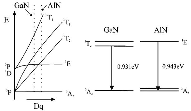
FIG. 3. Schematic Tanabe–Sugano diagram for a  $3d^2$  system together with the observed fine structure for the  $V^{3+}$  center in GaN and AlN. The larger crystal-field parameter  $Dq$  for AlN is caused by the smaller lattice constant of AlN compared to that of GaN and explains the different fine structure of the excited states.
