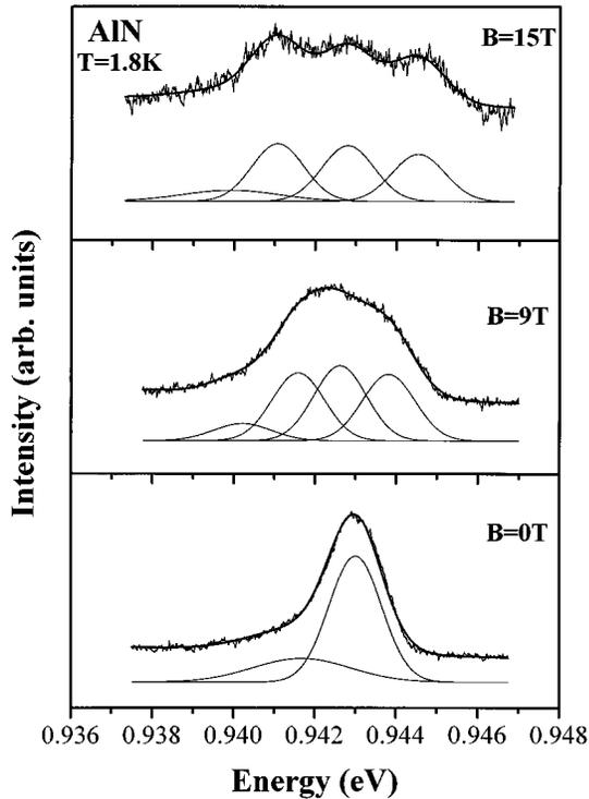
FIG. 1. Zero-phonon line region of the 0.943 eV emission in AlN for different magnetic fields at  $T=1.8$  K. The threefold splitting of the main ZPL is caused by the magnetic behavior of the  ${}^3A_2(F)$  ground state.
