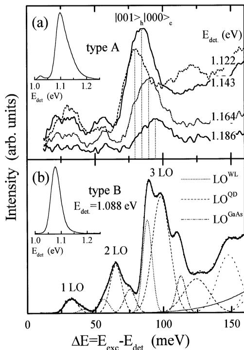
Fig. 1. PLE spectra for a type A sample with 5 QD layers and 36 ML spacer (a) and a single-layer type B sample (b). The insets show the respective PL spectra for GaAs barrier excitation.
