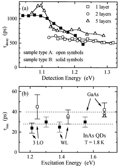
Fig. 3. PL decay (a) and rise (b) times derived from two-exponential fits of low excitation density PL transients for type A samples (open symbols) and the type B sample (solid squares).
