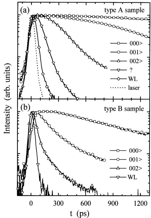
Fig. 2. High density PL transients of the ground and excited QD transition peaks for a 5 QD-layer type A sample with 20 ML spacers (a) and a type B sample (b).
